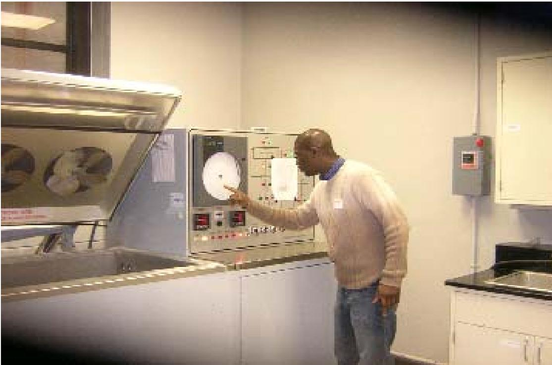
Fig. 3.8: Freeze and thaw chamber
