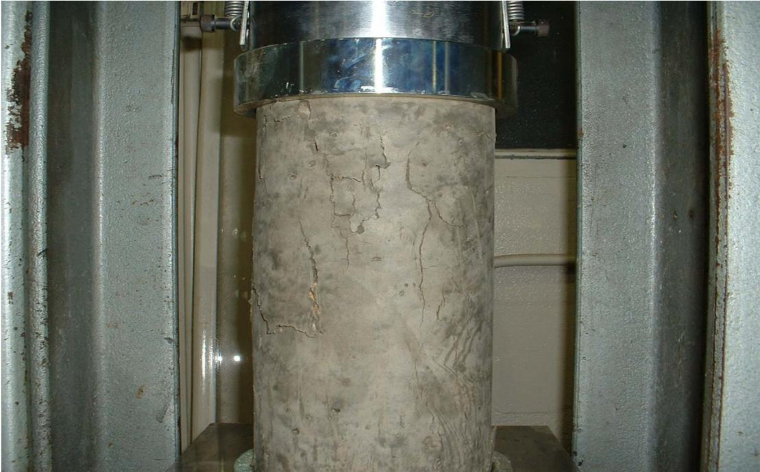
Fig.3.5: Specimen in the compression machine
