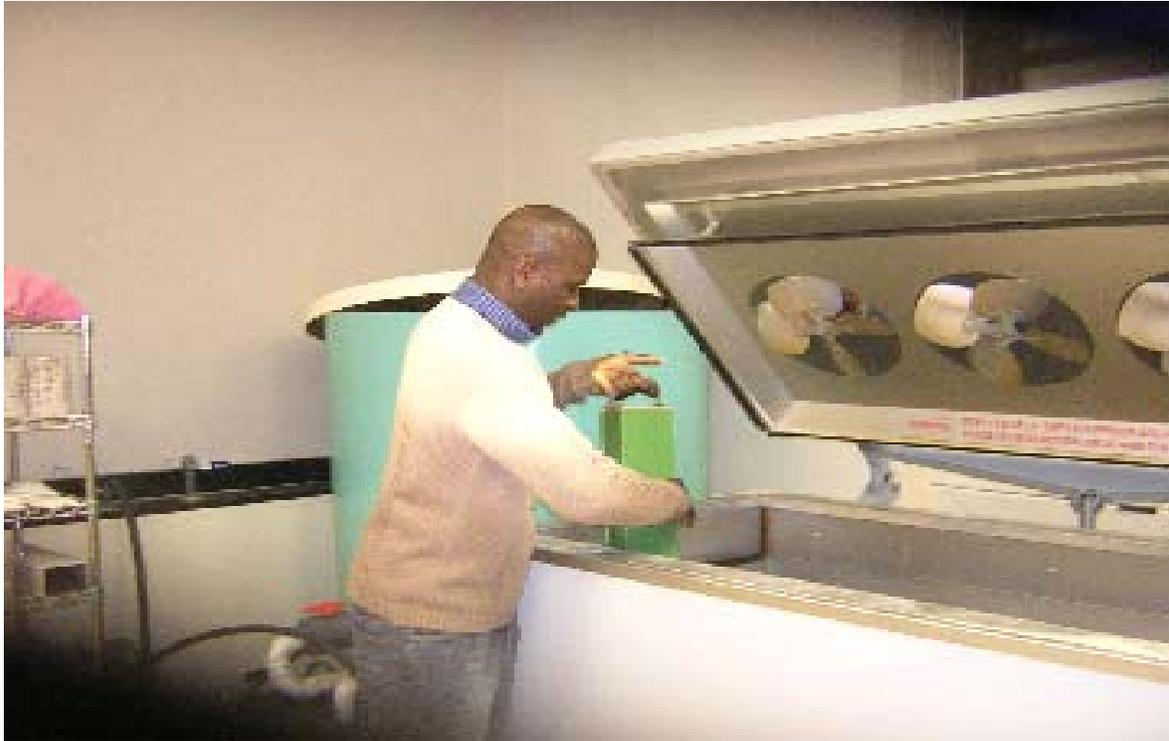
Fig.3.9: Specimen being removed from chamber for testing at thaw machine breakdown
