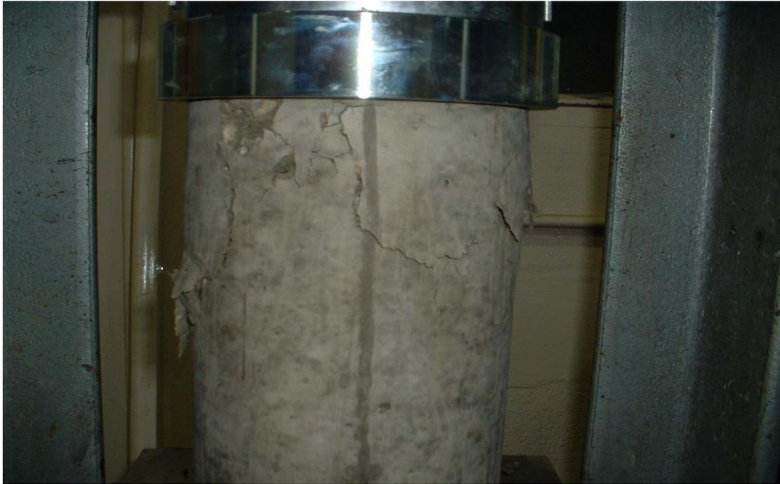
Fig. 3.6: Specimen under compression
