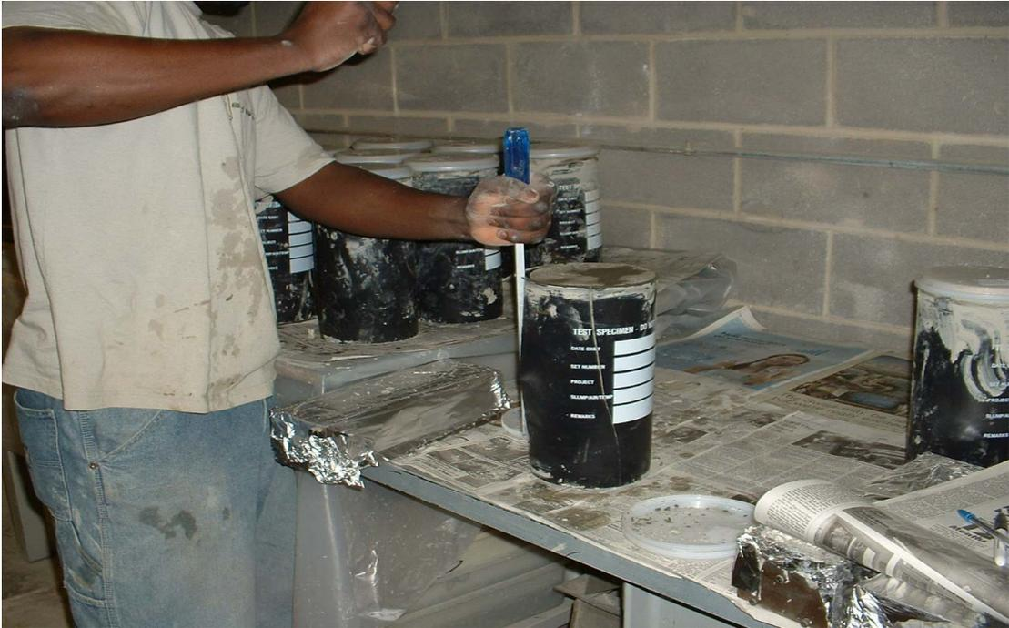
Fig.3.3: De-molding the cylindrical specimens
