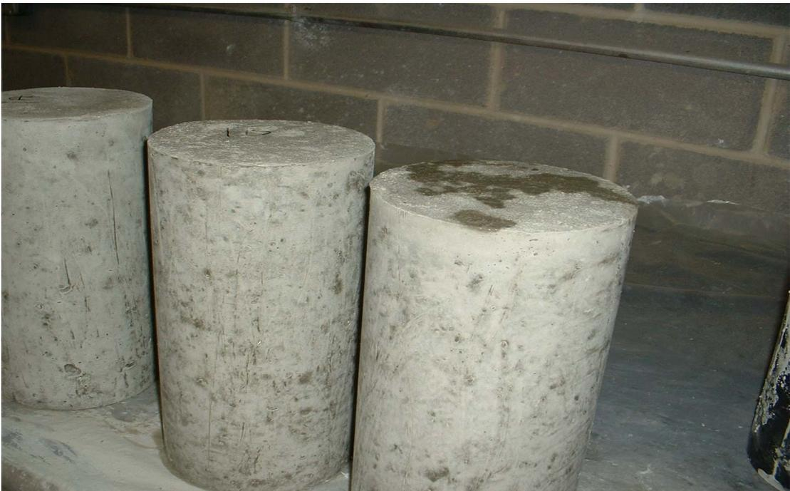
Fig.3.4: De-molded specimen for 4 hr compressive strength test
