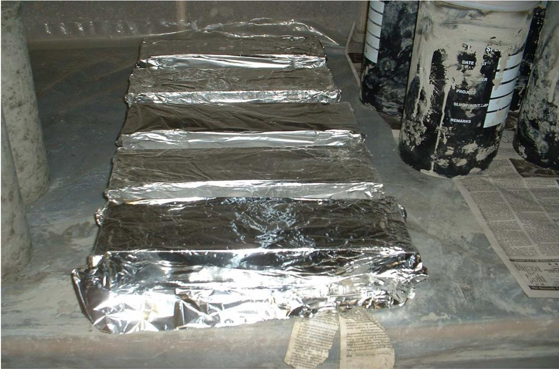
Fig. 3.7: Prism specimen covered with foil to prevent drying and shrinkage
