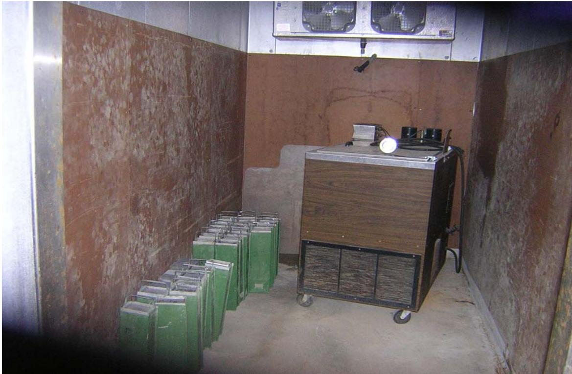
Fig.3.10: Storage Freezer used as storage facility during freeze and thaw failure
