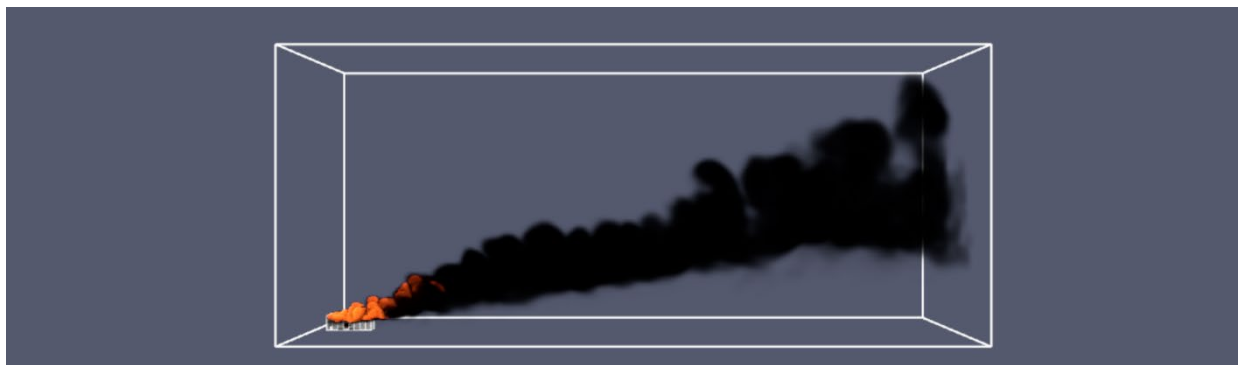
Figure 27. LFP non-flaming plume at 10 m/s, 22°C, and 2-hour duration
