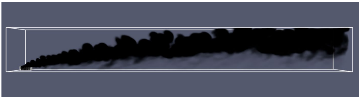
Figure 22. NMC non-flaming plume at 2 m/s, 22°C, and 0.5-hour duration
