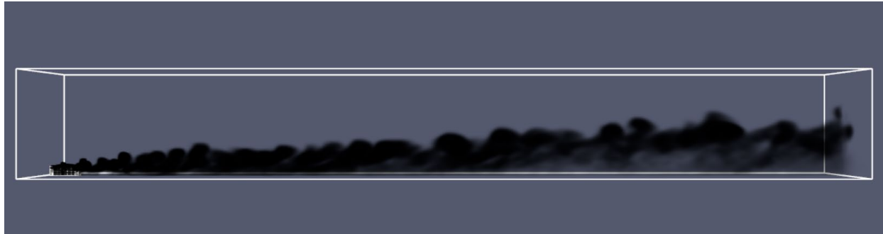
Figure 21. LFP non-flaming plume at 2 m/s, 22°C, and 6-hour duration
