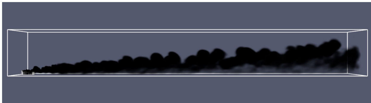
Figure 24. NMC non-flaming plume at 2 m/s, 22°C, and 2-hour duration
