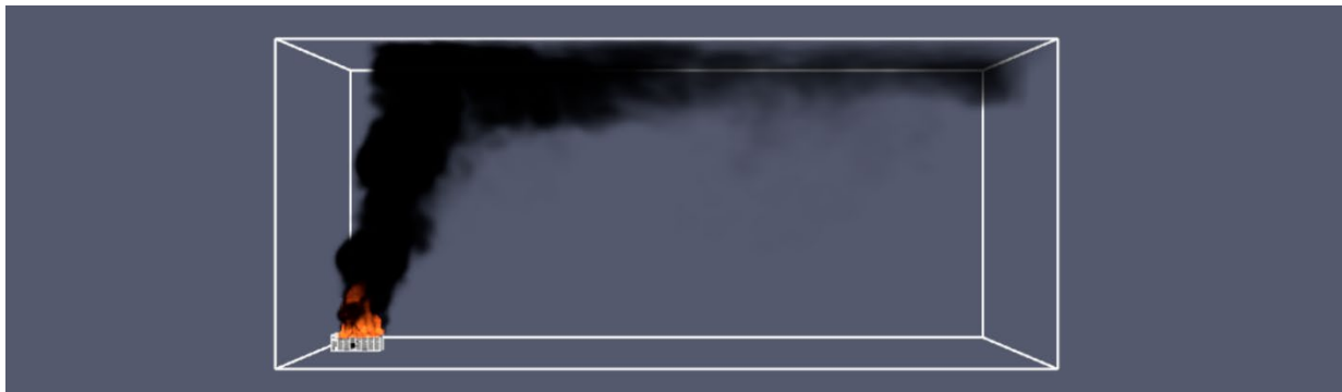
Figure 25. LFP non-flaming plume at 2 m/s, 22°C, and 2-hour duration
