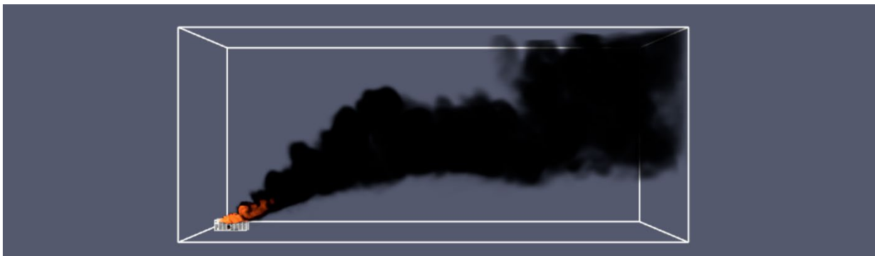
Figure 26. LFP non-flaming plume at 5 m/s, 22°C, and 2-hour duration
