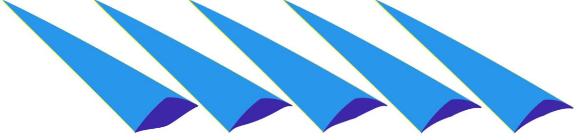
Figure 3.8: Analytical waverider constrained leading edge morphing geometries; left to right: fixed geometry, morphing geometries 1-4
