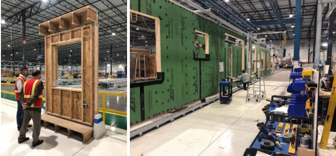
Figure 30 Internal assembly line of Blueprint Robotics
