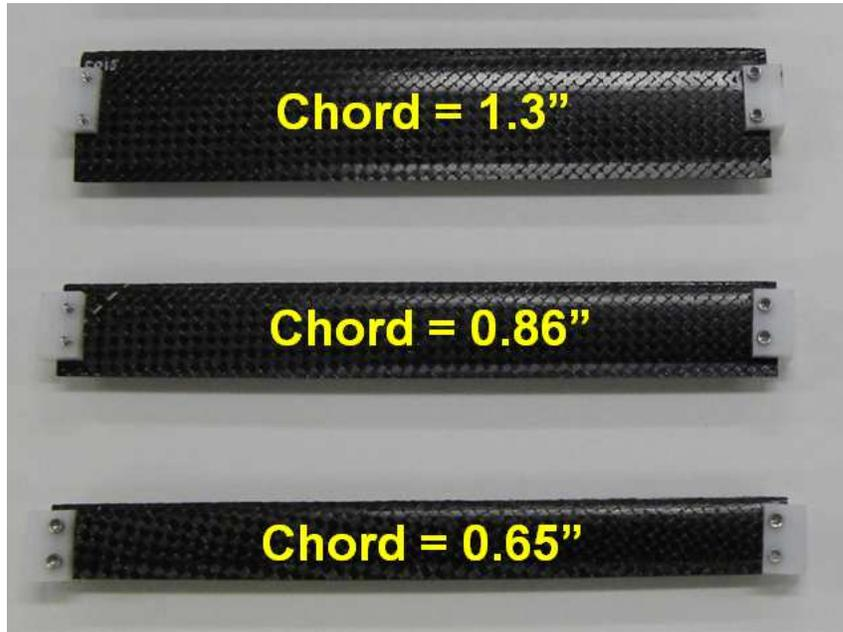
Figure 2.49: **Blades with different chord lengths.**
