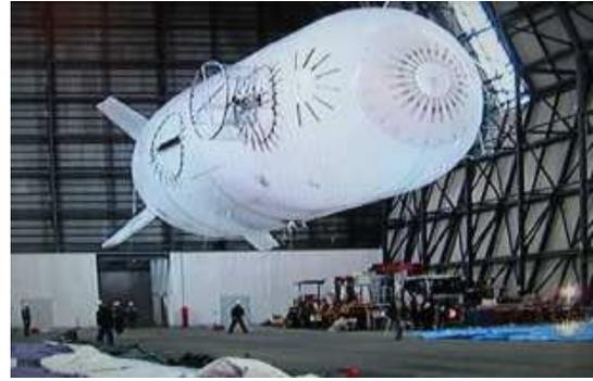
(b) Cyclorotors installed on a 20 meter airship.
