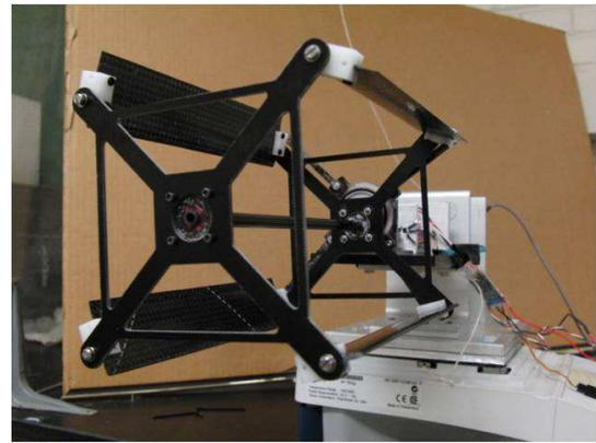
(b) Rotor used on the quad-cyclocopter.
