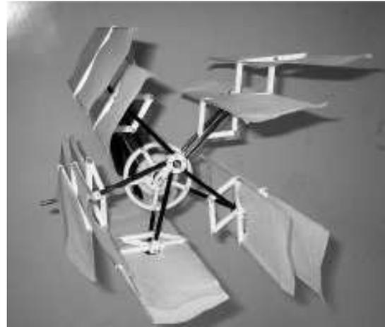
(b) Cyclorotor using the pantograph mechanism.
