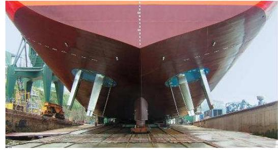
(b) Voith-Schneider propellers installed on a ship [35].
