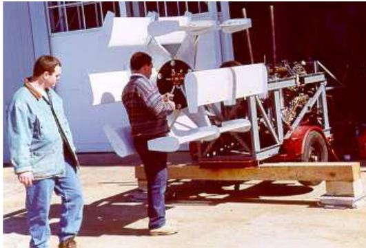
(a) Prototype cyclorotor [30].
