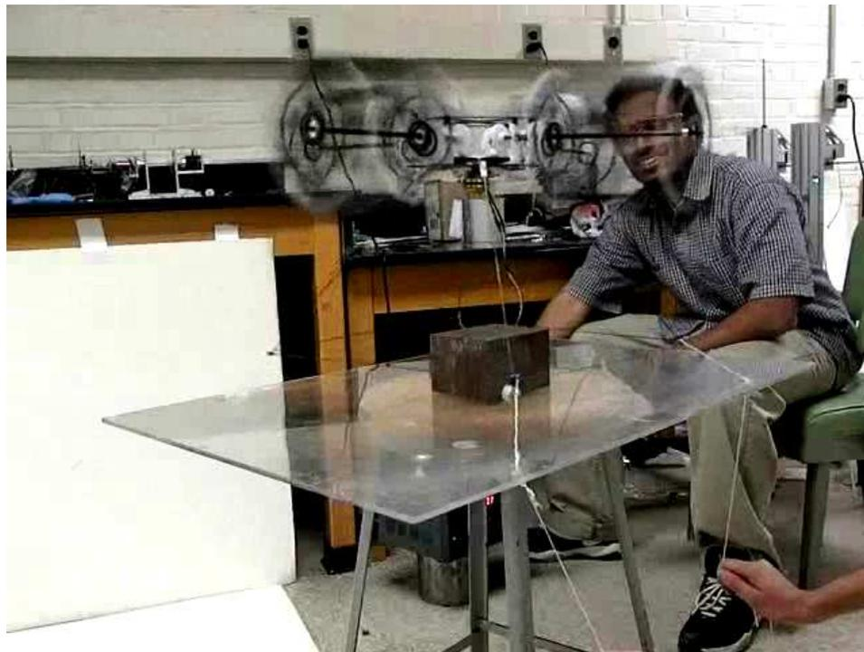
Figure 5.18: Tethered hovering of the quad-rotor cyclocopter.
