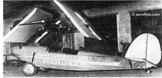
(b) Cyclogyro developed by Rahn Aircraft Corp (1935) [30].
