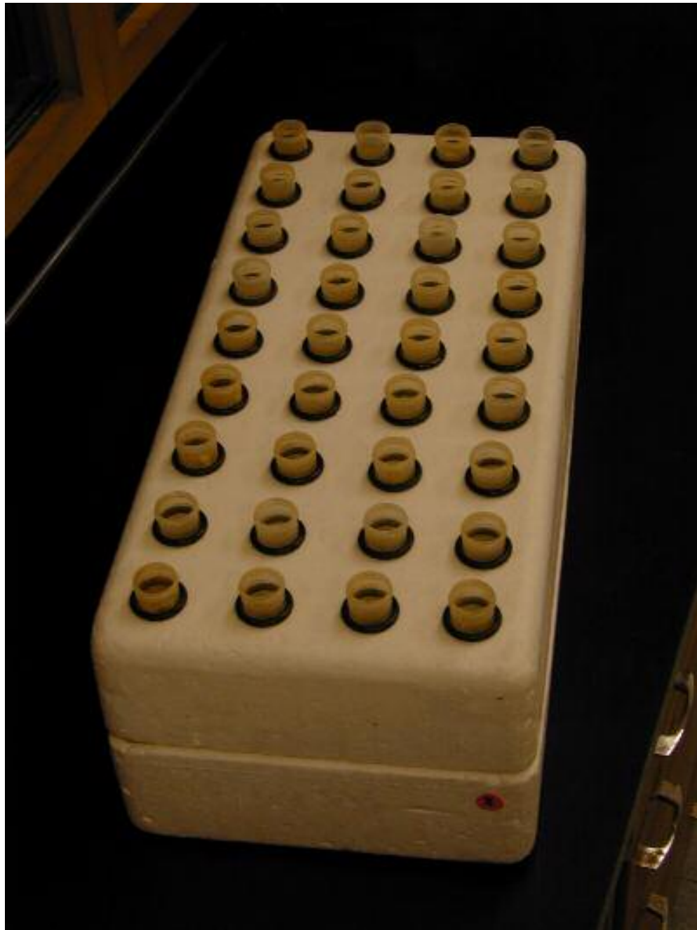
Figure 1. Image of the bioassay model of the Moisture Replacement System containing 36 grow tubes.
