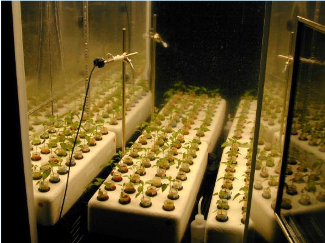
Figure 2. Image depicting arrangement of the three blocks (bioassay models of the MRS) within the growth chamber during the second trial.
