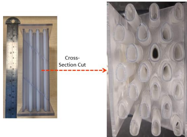
Figure 135: AOHX Small Test Print Section with Polyjet (Middle) Top View (Right) Overview
