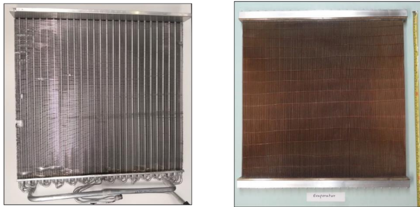
Figure 99: (Left) Baseline Fin-Tube Evaporator (Right) CNTHX-FS Prototype Evaporator (not to scale)
