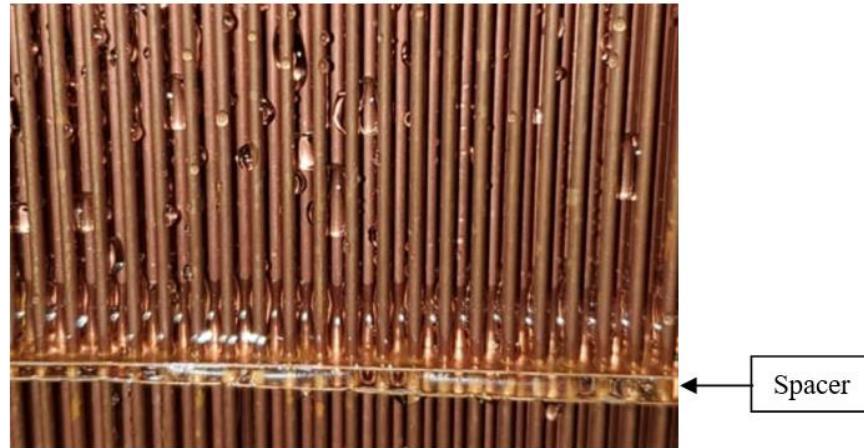
Figure 67: CNTHX1 Condensate Bridging during Wet Evaporator Testing
