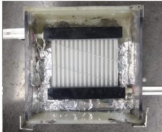
Figure 141: AOHX Mounted in Wind Tunnel Section for Radiator Testing (Air Inlet)
