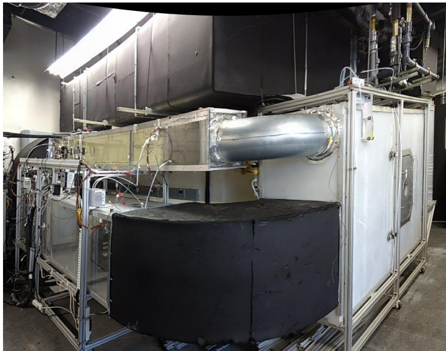
Figure 4: Heat Exchanger Test Facility, Closed Loop Wind Tunnel
