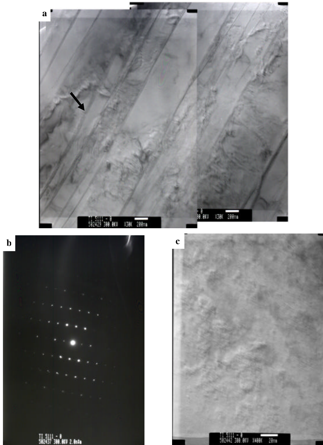
Figure 89: TEM images of FZ near the top center of the weld in Weld 0. (a) Image showing size of the parallel plates of Widmanstätten formed in the FZ. Note very thin remaining plates of \beta between the large \alpha plates as indicated by arrow. (b) Diffraction pattern from area shown in (a) indicating that the microstructure is Widmanstätten \alpha . (c) High resolution image from area (a) showing no particles exist in area.
