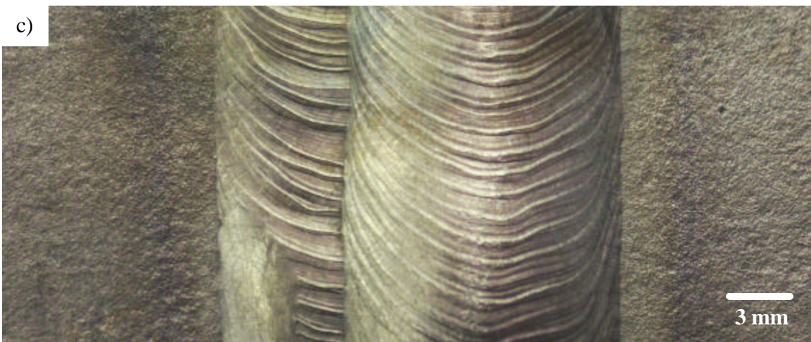
Figure 6: Optical pictures of weld zone surface of the FZ showing extent of surface rippling with increase in yttrium concentration. (a) Matching filler metal; (b) Modified 50 ppm Y filler metal; (c) Modified 200 ppm Y filler metal.
