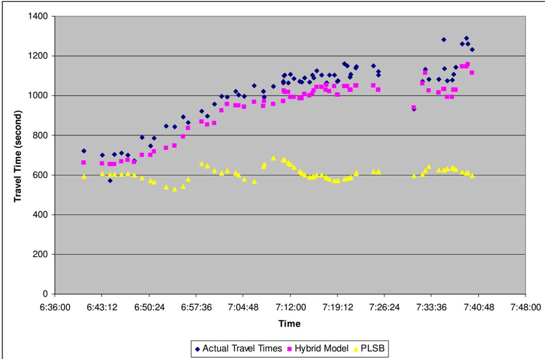
(a) Comparison between actual and estimated travel times in the subsegment from Detector 3 to Detector 10 on April 6<sup>th</sup>, 2006
