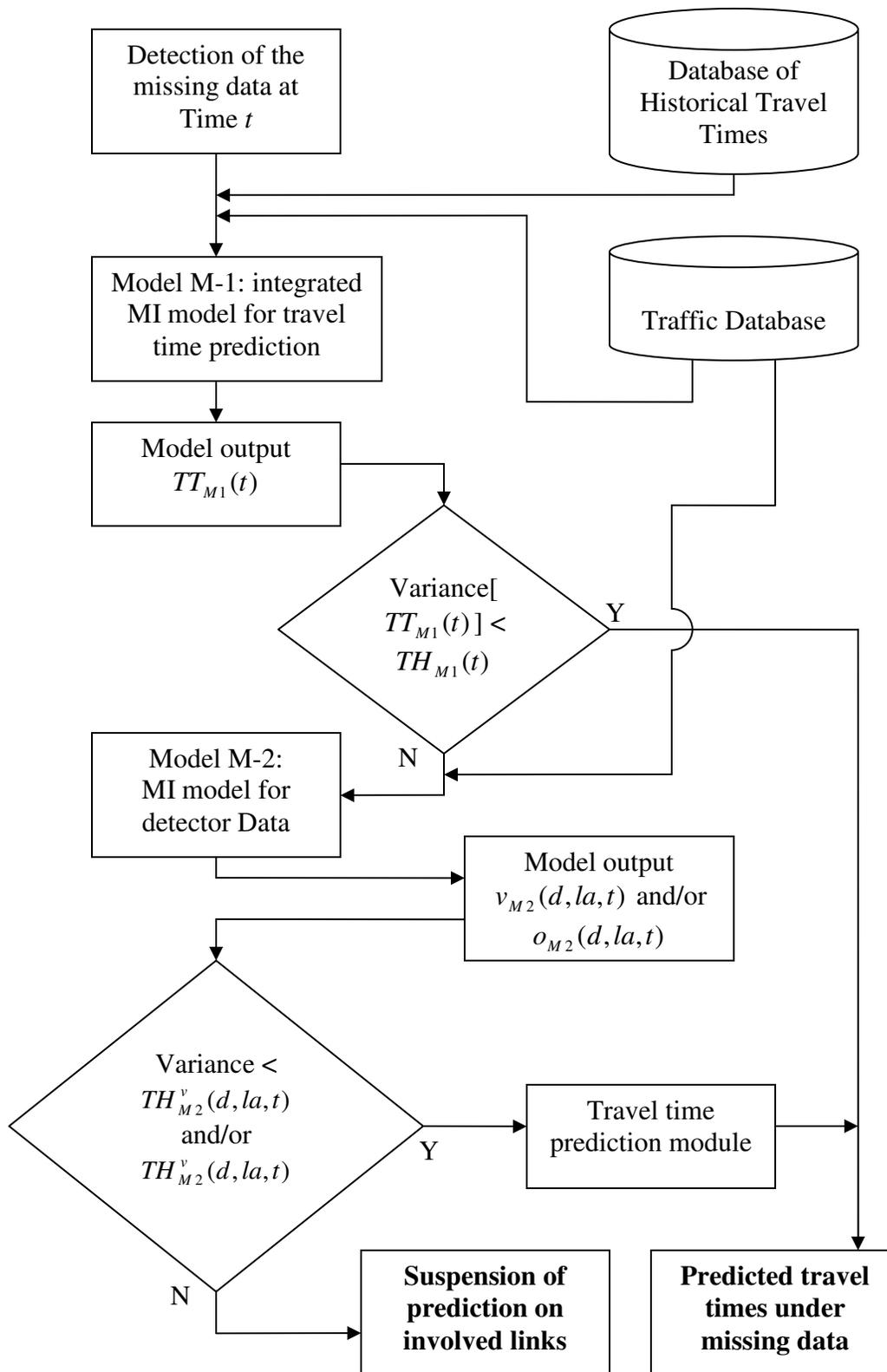
**Figure 6-3** Flowchart of the missing data estimation Module
