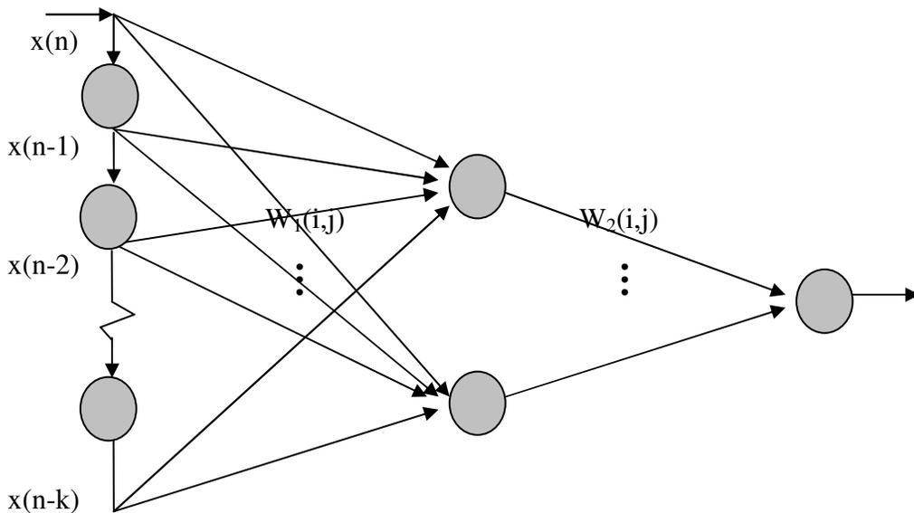
**Figure 2-1** Example topology of a Time-Delay Neural Network
