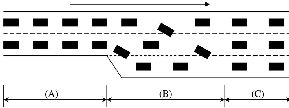
**Figure 4-2** Congestion pattern near a lane addition point
