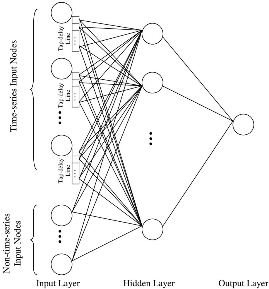
**Figure 5-2** Topology of the enhanced Neural Network that combines both time-series and non-time-series inputs
