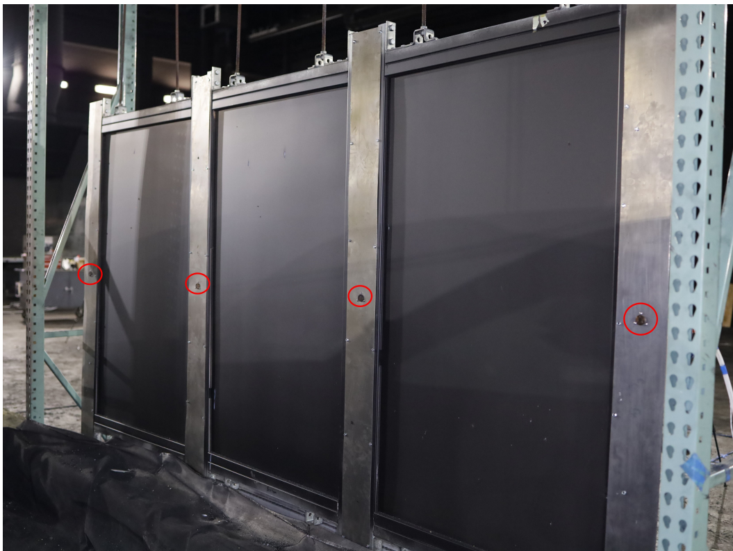
Figure 3.3: The red circles indicate the heat flux gauge placement on the panels.
