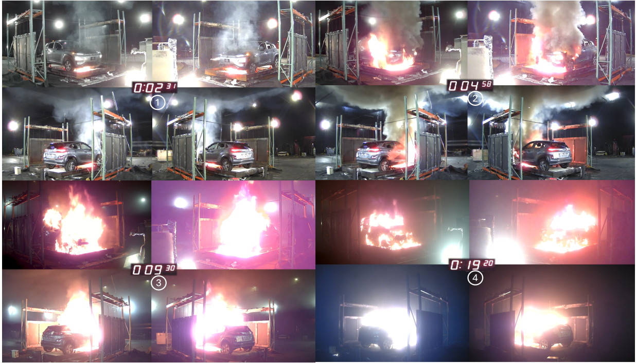
Figure 3.6: Still images of the experimental free burn at ignition onset of each major component. Image (1) is when burning under the vehicle begins, image (2) is hood ignition followed by image (3) cabin burning, lastly image (4) with the rear portion of the vehicle igniting. Each quadrante of images displays one section of burning from four distinct angles with the corresponding time in minutes located at the center of the quadrant.
