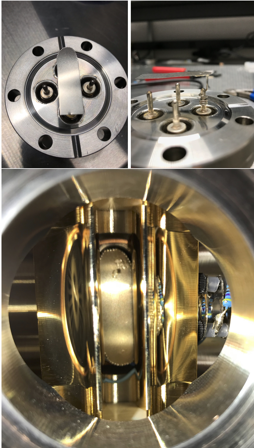
Fig. D.4: Photos showing the collector plates used in the 90^\circ deflector experiments. (Top Left) Collector plate was made from nickel shim stock and mounted onto a CF electrical feedthrough, allowing measurement of ion current onto the nickel plate. (Top Right) Side view showing mounting setup of nickel plate. A rigid wire was soldered to the plate, keeping it in place during experiments and connecting the plate to the feedthrough. (Bottom) Photo of the collector plate in place inside the interface chamber. An identical collector plate and CF feedthrough setup was installed on the opposite side of the 90^\circ deflector as well.
