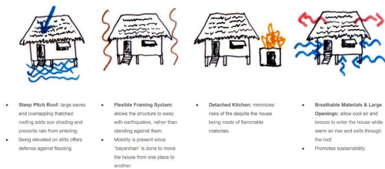
Figure 70. Passive Cooling Design (Source: drawn by author)
