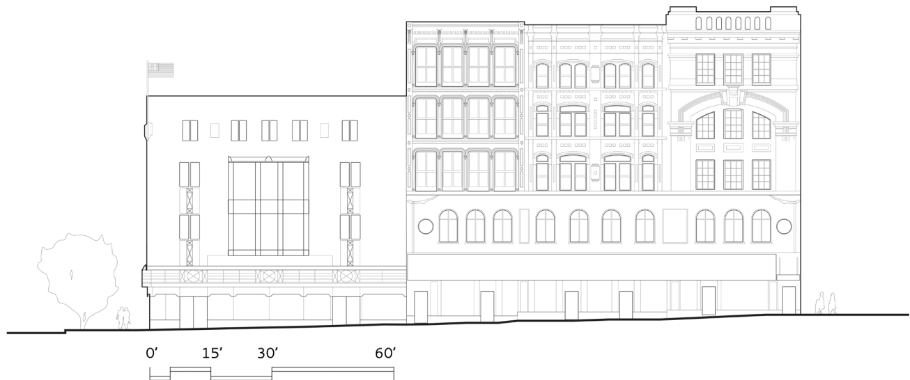
Figure 21: North Howard elevation of proposed design of new museum building with restored and preserved facade. Illustration by author.
