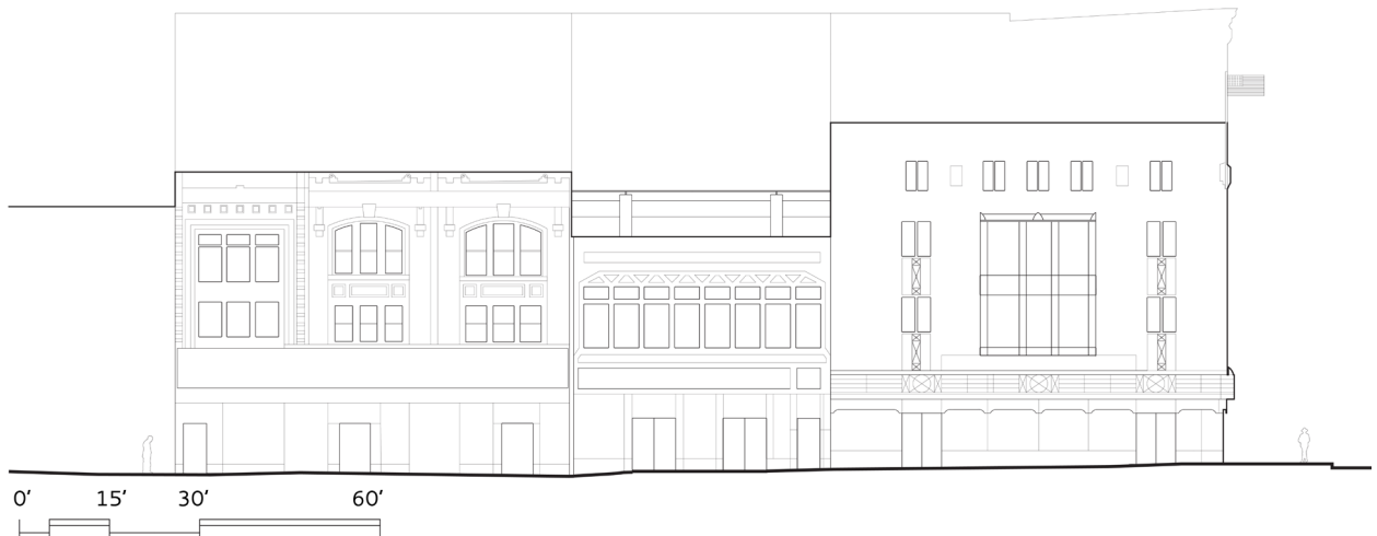
Figure 20: West Lexington elevation of proposed design of new museum building with restored and preserved facade. Illustration by author.
