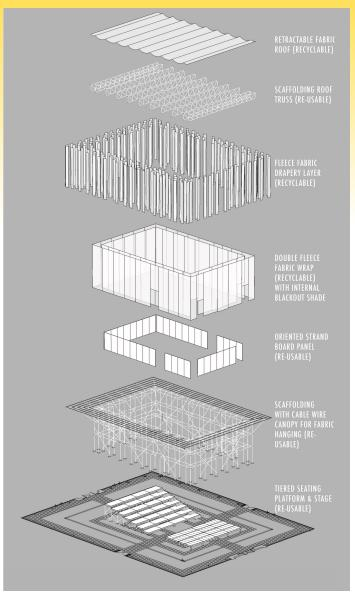
demonstrating how temporary structures can be added to a permanent floor plan.
