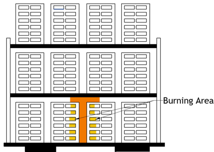
Figure 39 Schematic illustration of burning area identification for plastic pallet commodity based on video analysis.
