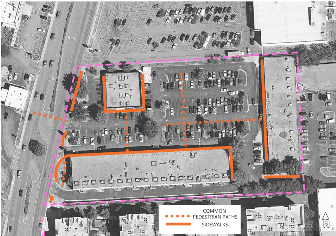
Figure 42: Sidewalks are not aligned with desired pedestrian routes at the project site. Source: Garlow, 2026
