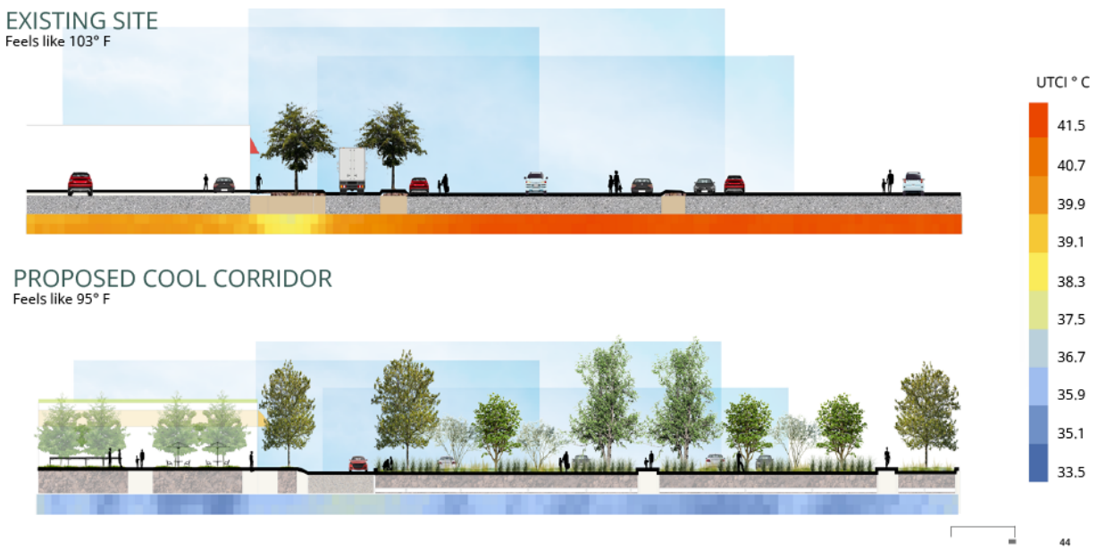
Figure 92: Comparison of UTCI along proposed cool corridor in existing versus proposed design. Source: Garlow, 2026
