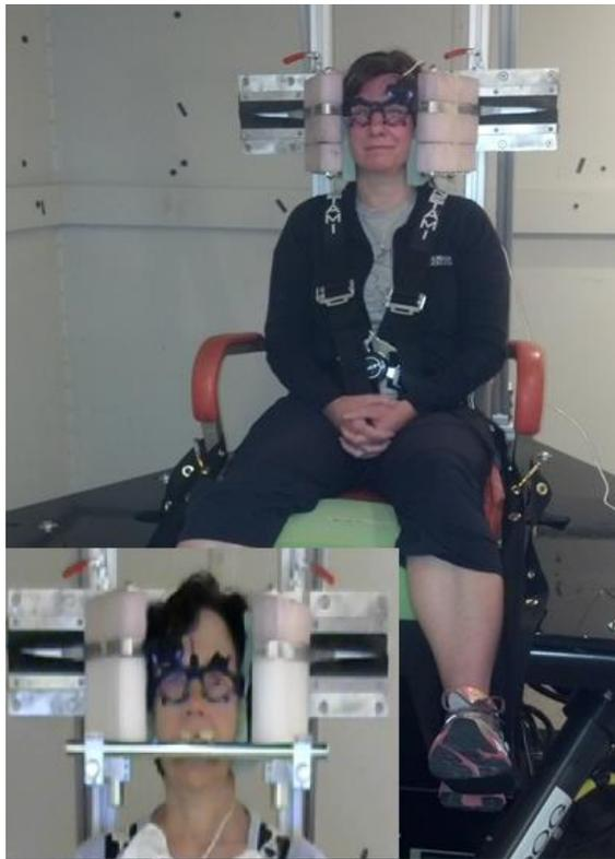
Figure 6-3. Picture of the experimental set-up for the “seated walking” portion on the MOOG. The bite bar and head restraint are shown in the inset.
