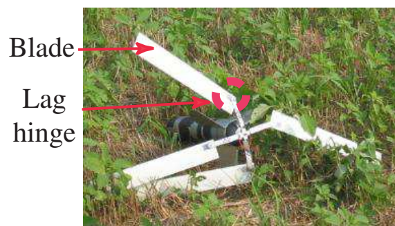
Figure 5.23: Lag hinge increases blade survivability on impact.
