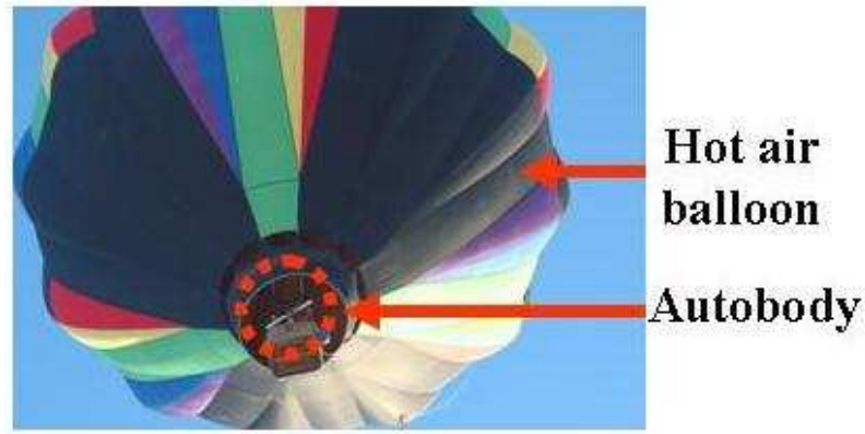
Figure 5.12: Autobody instrumented drop test performed from a hot air balloon.
