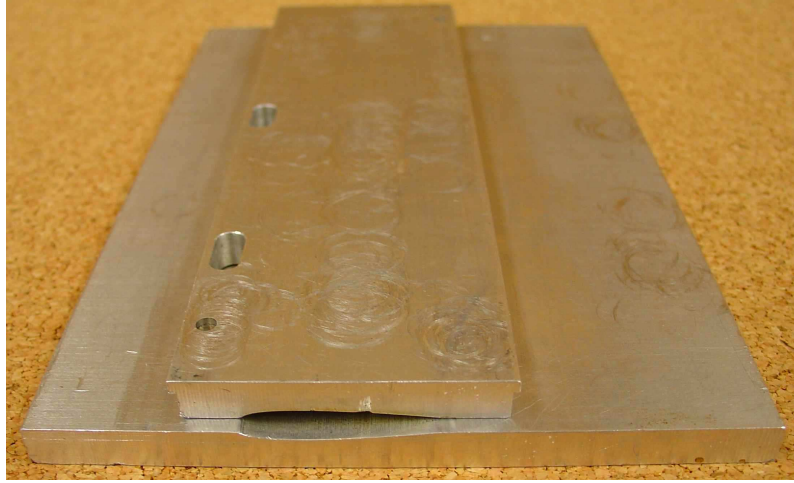
Figure 4.5: NACA 0010 mold used to manufacture the small scale blades.
