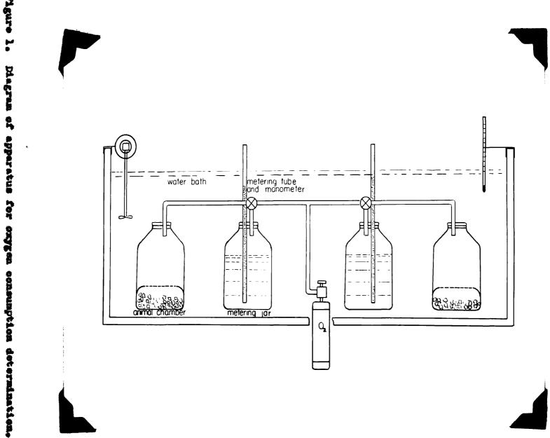
screening for the absorption of carbon dioxide. The soda lime was changed each day and agitated vigorously after every run. The entire apparatus was tested for leaks overnight, after each day's runs.
