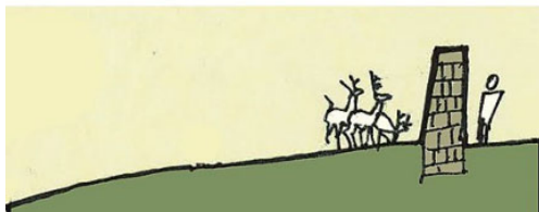
Figure 36: Cartoon displaying what a ha ha is and why it can be used (Photo Cred: Wikipedia)
