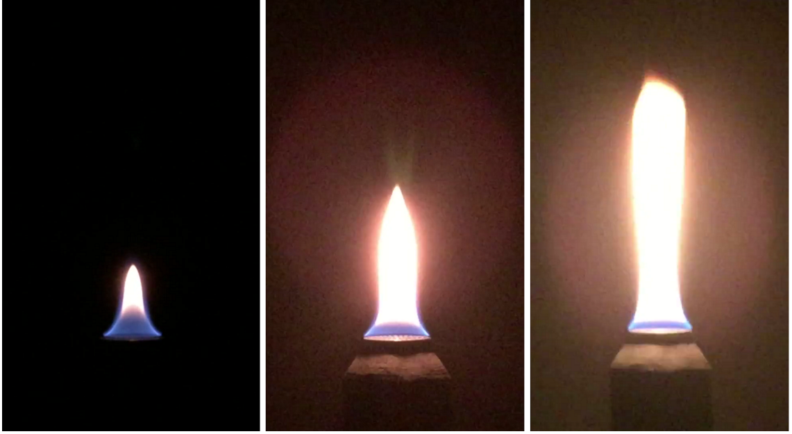
Figure 2.8: Flames for the 25 mm BRE3 burner with mass flow rates of 4 \text{ g/m}^2\text{-s} (left), 8 \text{ g/m}^2\text{-s} (center) and 12 \text{ g/m}^2\text{-s} (right).
