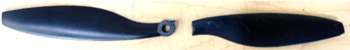
Figure 3.10: Broken Forum 79 10x4.5 propeller that failed during propeller-driven rotor operation.
