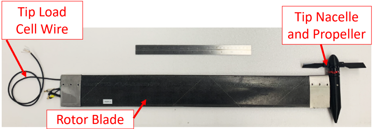
Figure 3.22: Composite rotor blade and tip propeller and load cell used in rotor-propeller hover loads experiment.
