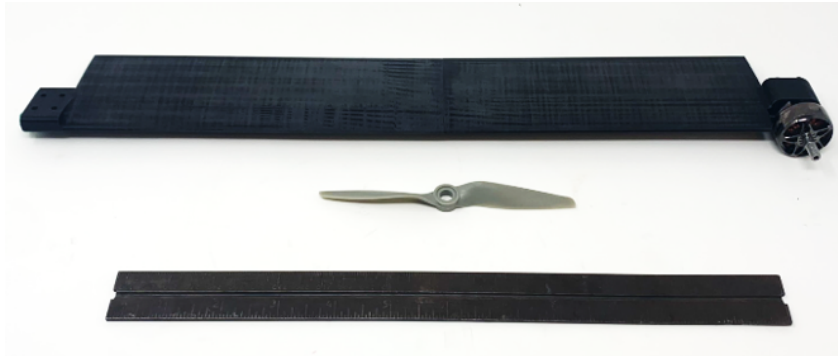
Figure 2.4: The 14 inch span, 3D printed propeller-driven rotor blade.
