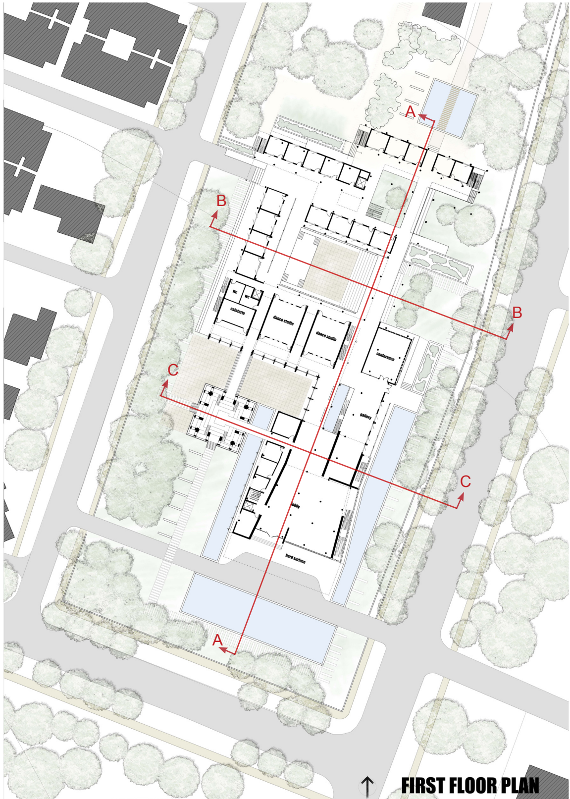
Fig.44 First floor plan of performing arts center. The circulation flows through series of closed, semi-closed and open spaces. Also they are located on the perimeter so that the living spaces can be buffered from the sun.
