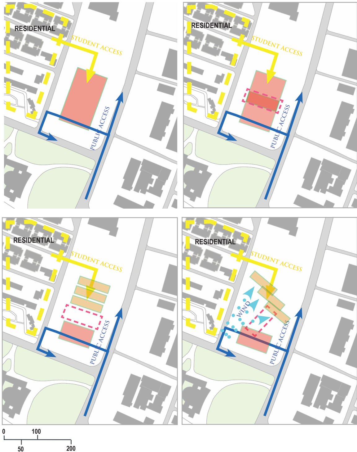
Fig.42 Diagram showing site analysis with respect to land use and climatic analysis. The prevailing winds are from the SW direction during the summer months thus the building mass is broken into smaller bar buildings that allow air to circulate more freely through the spaces.
