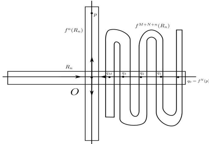
Figure 2.6: The construction of a horseshoe.
