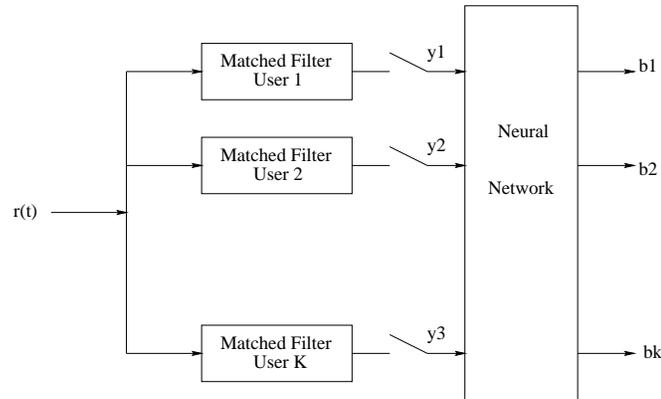
Figure 4.6: A neural network receiver for multiuser demodulation
