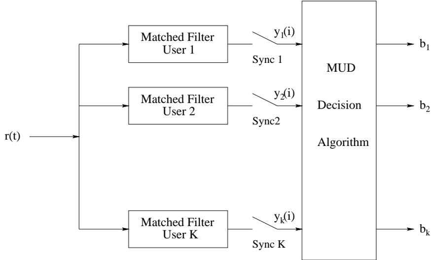
Figure 4.5: The general structure of multiuser detection(MUD)
