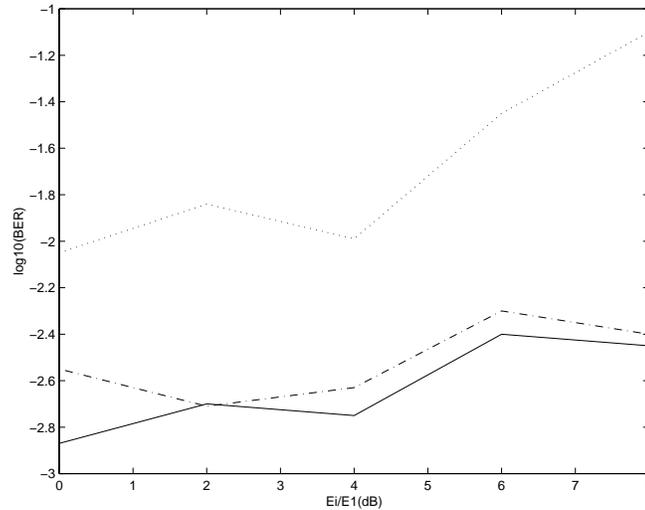
Figure 5.14: Bit error rate versus  $E_i/E_1$  for 5-user channel with the SNR of user 1 fixed at 8dB, where the solid line is OMD, the dash-dot line is the SRN and the dotted line is the MLP.
