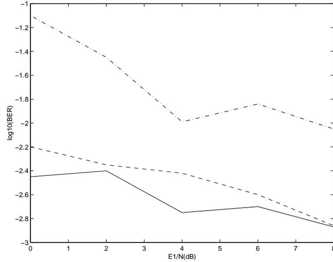
Figure 5.13: Bit error rate versus  $E_1/N$  for 5-user channel with the SNR of the other users fixed at 8dB, where solid line is the OMD, the dash line is the SRN and the dash-dot line is the MLP.
