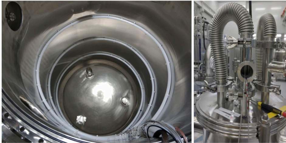
Figure 5.18: The three PVC calibration tubes attached to the OV (left) and the handling port (right) to load the calibration sources in the workspace.
