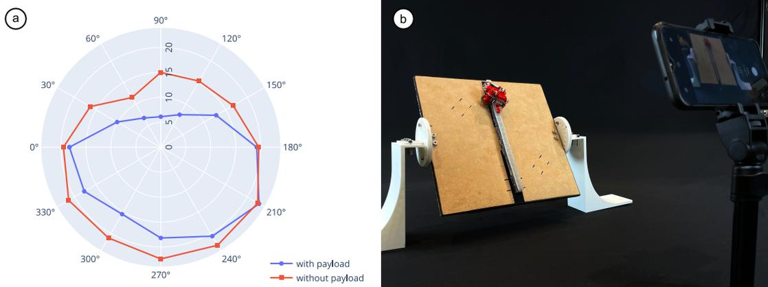
Figure 4.1: a) Speed in  $cm/s$  with and without a payload (20gm) plotted against approach angle. b) Test setup used to test the speed with and without a payload.
