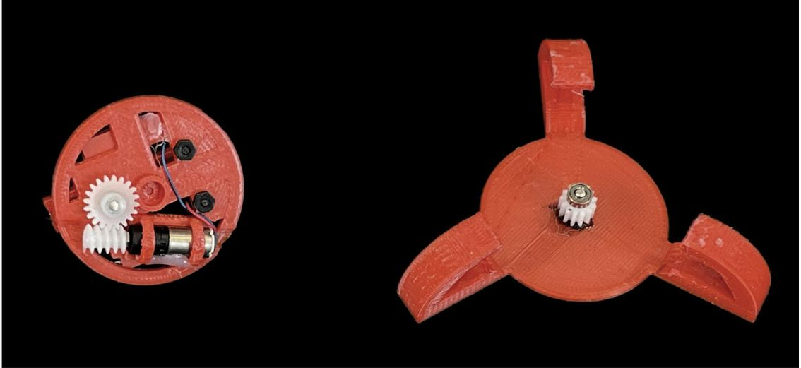
Figure 3.9: The turntable mechanism. When the bot makes contact with the copper pads on top and sends a signal through the motor driver, the rotor rotates around the base, which also rotates the bot.
