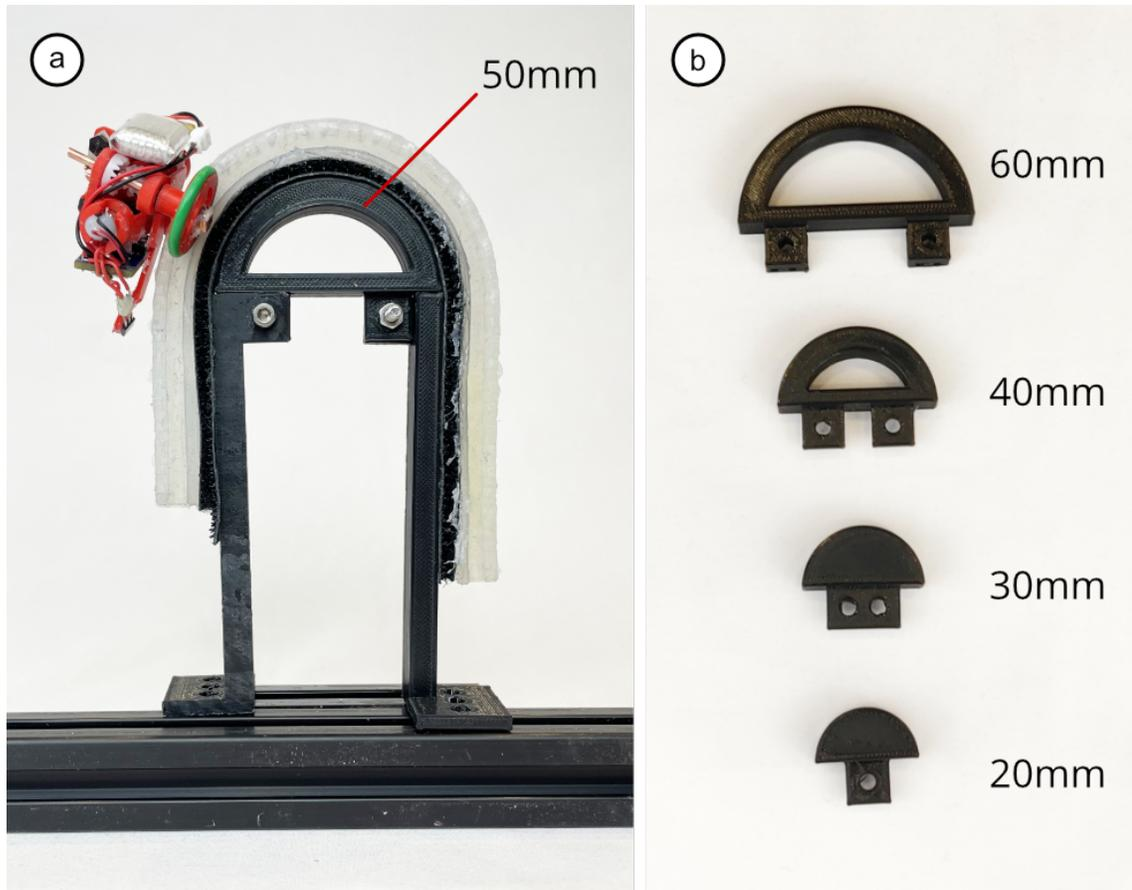
Figure 4.2: a) Test setup to determine the minimum rigid curve that can be traversed by Calico. b) Different curvatures used.
