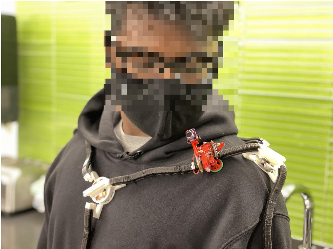
Figure 5.3: Calico positions itself near the neck of a user to transmit audio.
