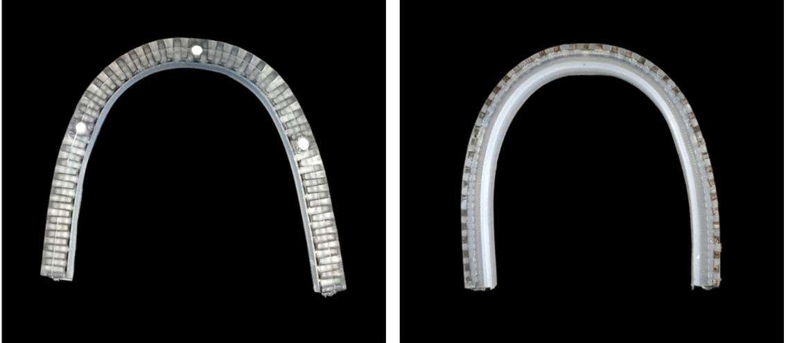
Figure 3.6: Due to the live-hinge design, the track can be flexed in all directions while still restricting the degree of freedom to keep the wheels of the bot in the crevice.
