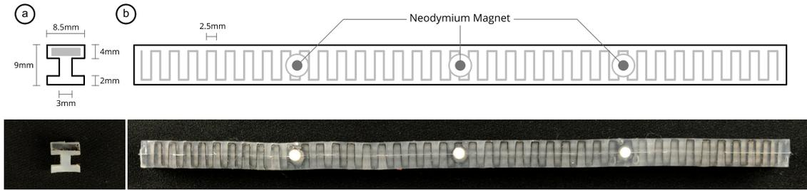
Figure 3.5: Meta-material track design. a) Cross-section of the track. b) Top view of the track with embedded magnets and a live-hinge pattern of the inlay.
