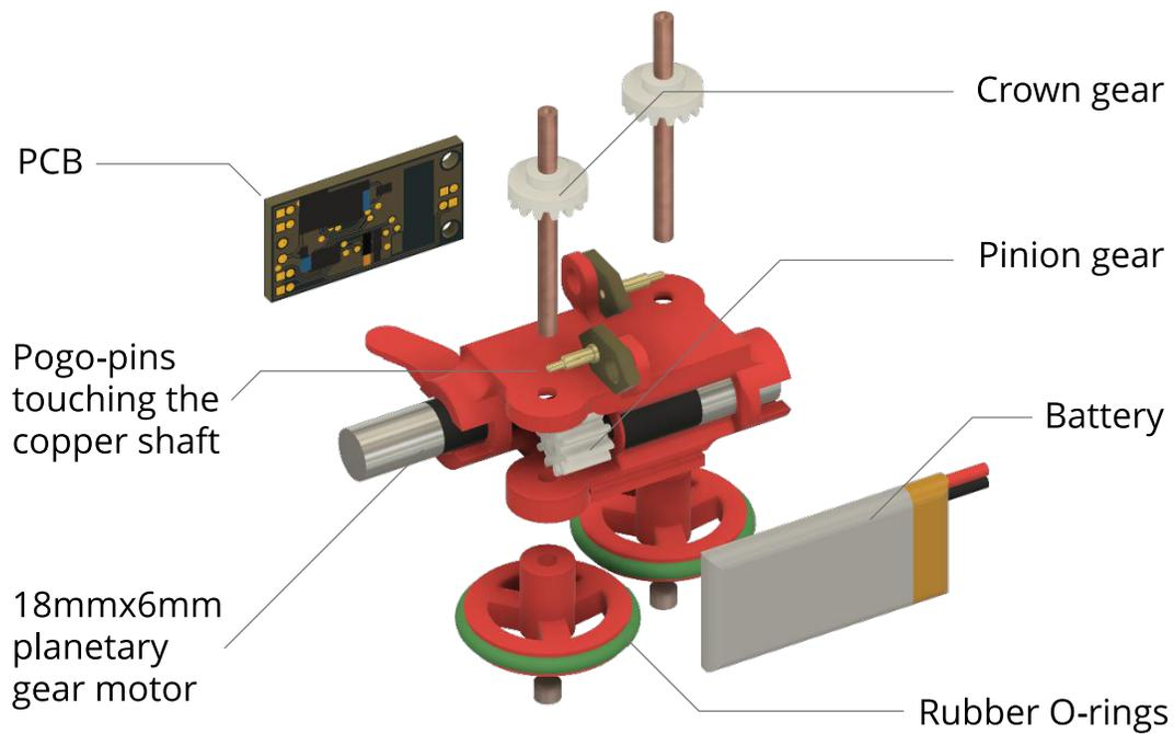
Figure 3.3: An exploded view of Calico
