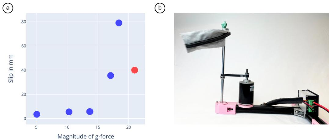
Figure 4.3: Testing the slip of the device when subjected to different g-forces. a) Scatter plot showing the slip vs the g-force encountered. At 21g (marked in red), the wheels broke through the inlay instead of slipping along the groove in the track. b) Test setup used to run the experiment.
