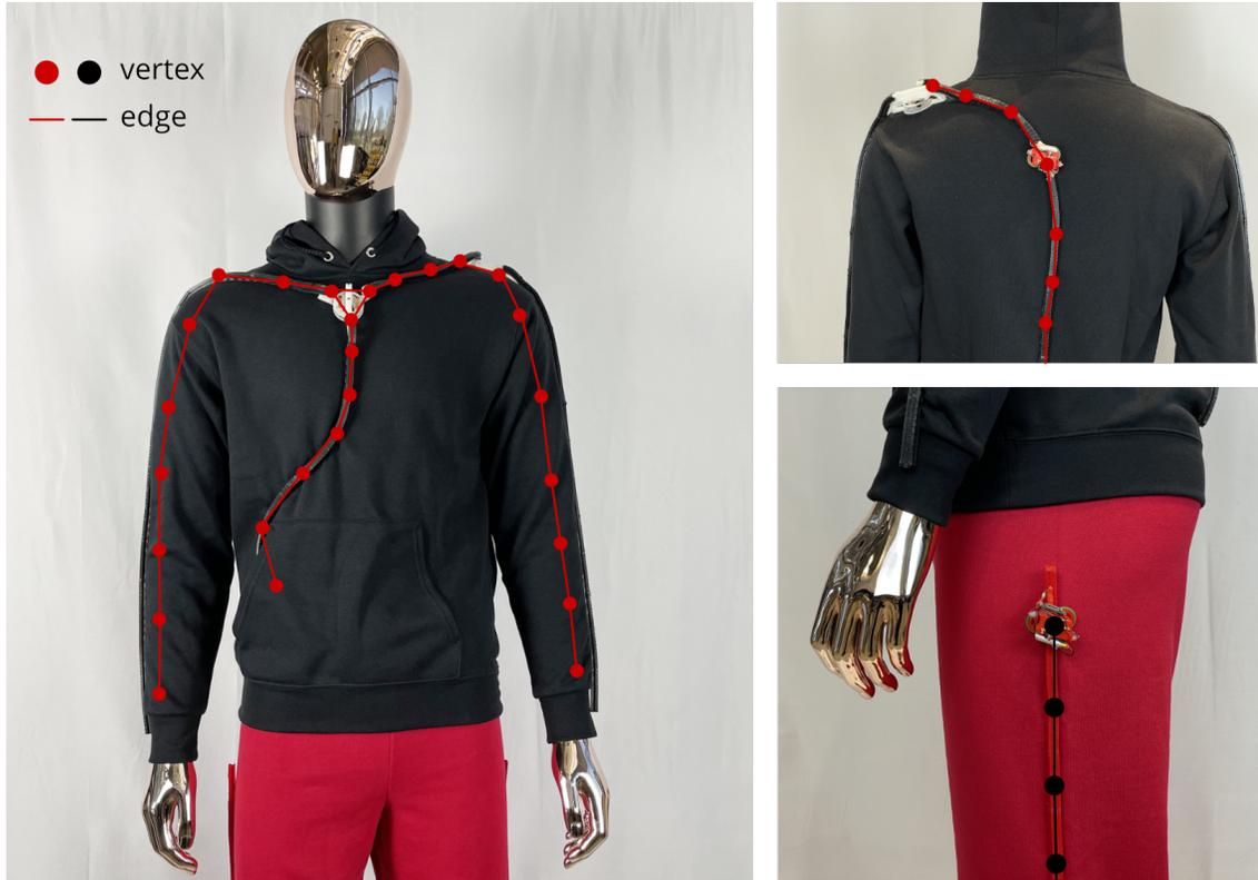
Figure 3.10: Using a track system on the clothing allows us to project the 3D terrain onto a 2D graph structure. The points of interest must be chosen before this projection.
