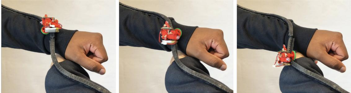
Figure 5.6: Using magnetic connects at the end of the track, Calico can move from one user to another. This functionality can also be extended to other surfaces.
