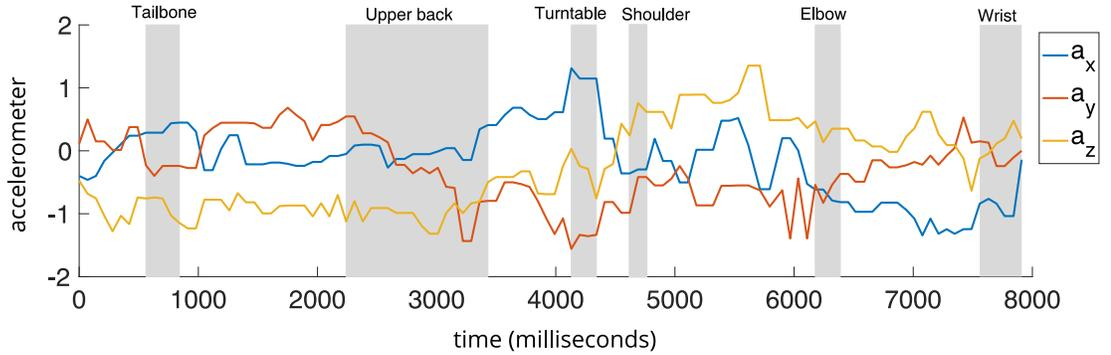
Figure 6.1: The median filtered accelerometer time series data collected during a full body auto calibration step for precise anatomical localization.
