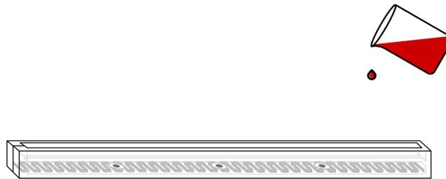
Pour into mold with the inlay and placeholders for magnets
