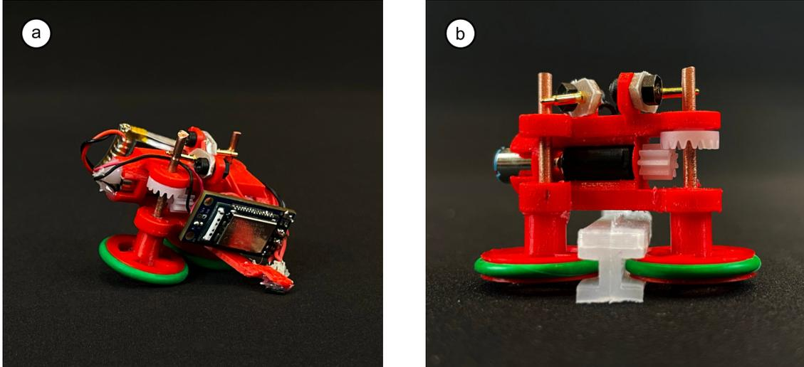
Figure 3.2: a) The Calico bot. b) The latching mechanism used by the Calico bot to move along the track.
