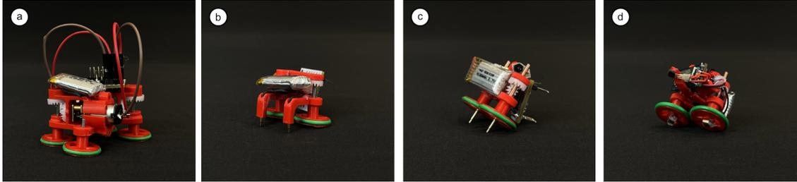
Figure 3.1: The different design iterations of Calico. a) The proof-of-concept with 4 wheels and 2 Pololu Micro Metal Gearmotors. b) Switching to a smaller motor with a different gear assembly. The overhangs would easily get caught on wrinkles in the clothing. c) Switching to a copper shaft to avoid the overhangs but still create electrical contact with the turntable. d) Switching to dual motor drive and magnets with copper plates to increase the speed and the climbing capacity.
