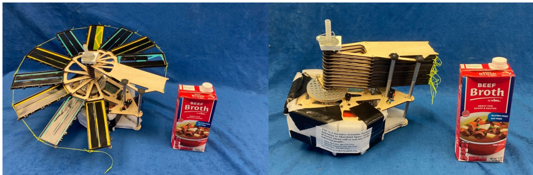
Fig. 4 (left to right): 1) CATITO v2 in deployed position after payload recovery. 2) CATITO v2 in retracted position after payload recovery. (Beef broth for scale)
