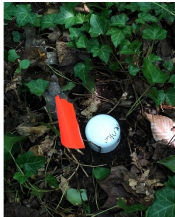
Figure 9. An example of an in situ soil incubation using a 5.08 cm diameter capped PVC pipe tapped 12.70 cm into the soil. This sample was taken at an urban forest patch plot located at Johns Hopkins University Homewood Campus (plot JHU 26) in Baltimore City, MD (Figures 3 & 5). This method was used alongside an unincubated soil sample to determine the rates of N mineralization and nitrification by measuring the change in \text{NH}_3\text{-NH}_4^+ and \text{NO}_2^- - \text{NO}_3^- concentrations over the time of the incubation (from September 16-18, 2022, to October 16-17, 2022).
