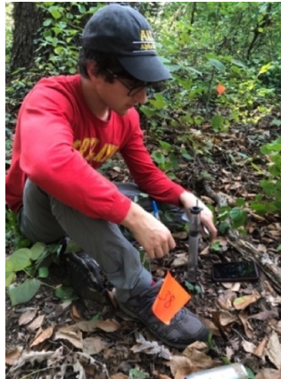
Figure 8. A field volunteer, Benjamin Robinson, using a Mini Disk Infiltrimeter made by METER Group (Pullman, WA, USA) on a random, flat point cleared of leaf litter at a plot in an urban forest patch located at Johns Hopkins University Homewood Campus (plot JHU 22) in Baltimore City, MD (Figures 3 & 5). This instrument is used to estimate unsaturated hydraulic conductivity by measuring the amount of water which transfers from the device into the soil through a porous stainless-steel disk over time, with a set suction. Suction was set to two cm and volume was recorded every 30 s until seven to 15 mL of water seeped into the soil.
