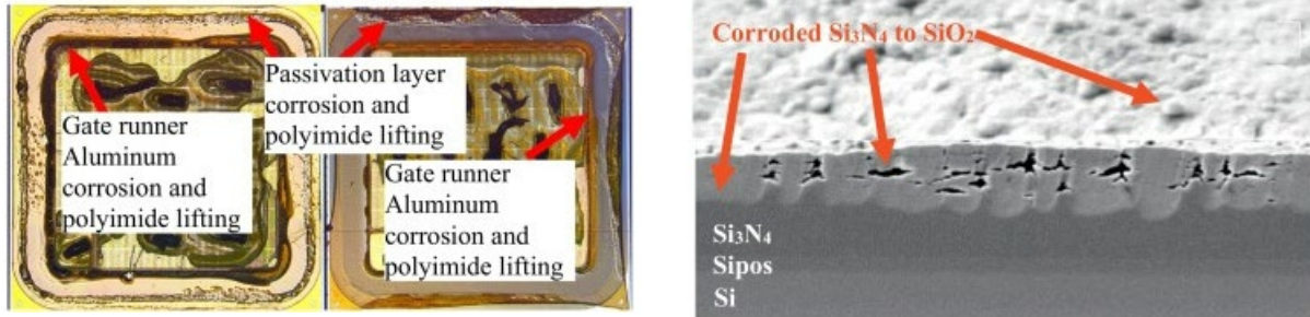
Figure 6: Failure in Silicone gel encapsulated silicon nitride IGBT module
