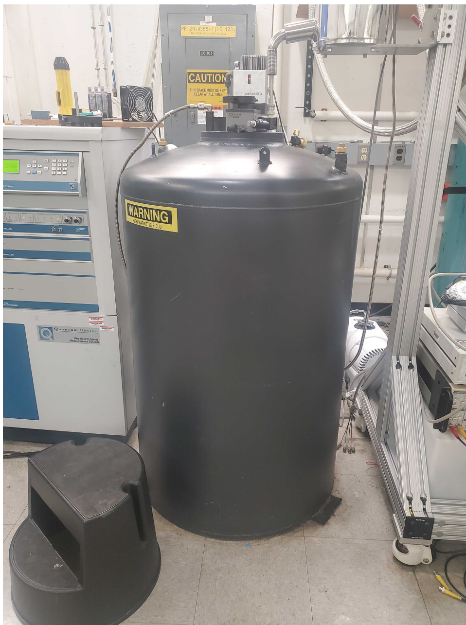
Figure 2.7: Quantum Design 14T PPMS system used to complete high pressure electrical transport measurements of \text{Ba}_{1-x}\text{Sr}_x\text{Ni}_2\text{As}_2 . Electrical transport apparatuses of measurement interest are loaded from the top down a thin cylindrical chamber. The sample environment is then purged and sealed at vacuum before beginning measurements.
