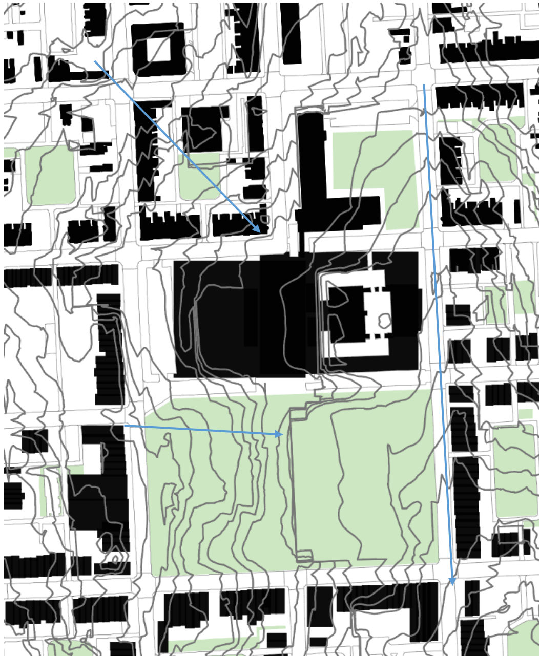
Fig. 49. Blue arrows mark the direction of water flow on the site. There is an 18-foot elevation difference from the west to the east side of the school site. By Author, 2020.
