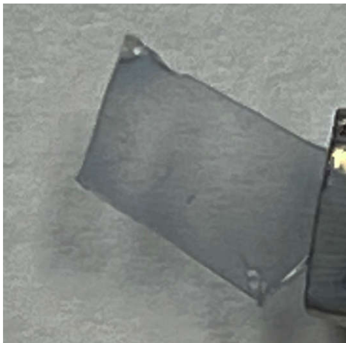
Figure 5.3. Photo of typical chiral Au-CdS thin films for low temperature optical spin measurements
