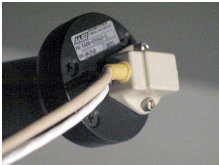
Figure 58: Underside of Wand Showing Sensor and Connection to Onyx2
