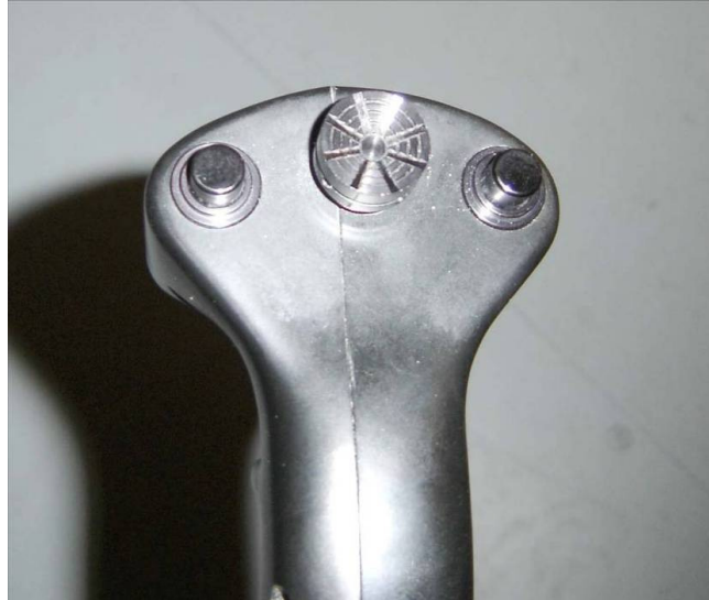
Figure 57: Back View of Wand Showing Joystick and Buttons 2&3
