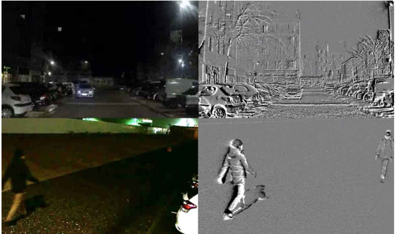
Figure 3.15: Sourced from Prophesee, the figure shows how a regular RGB camera compares to an Event camera, which fundamentally sees the world as events in asynchronous time that occur at specific pixel locations. Each pixel in an event camera asynchronously produces an event when pixel intensity sufficiently changes sufficiently quickly, labeling that row and column pixel with a timestamp of the event.
