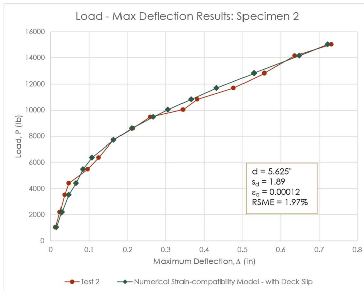
Fig. 4.26(a) Load-deflection model comparison with test specimen 2.
