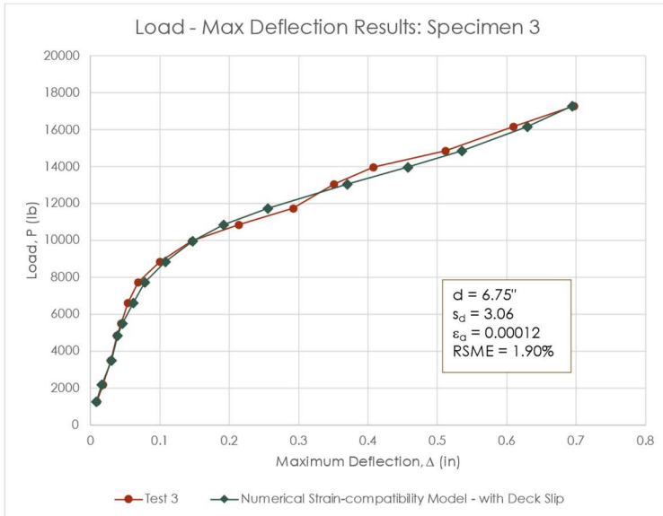
Fig. 4.26(b) Load-deflection model comparison with test specimen 3.
