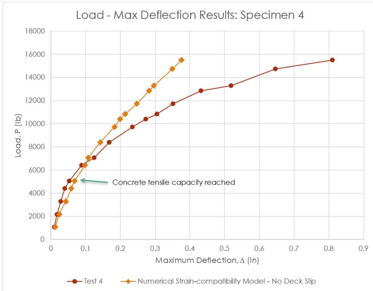
Fig. 4.22(c) Load-deflection model with no slip comparison with test specimen 4.
