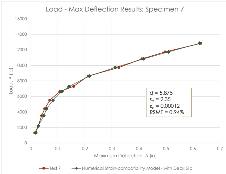
Fig. 4.26(f) Load-deflection model comparison with test specimen 7.
