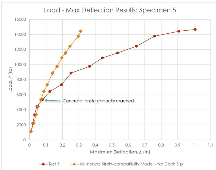
Fig. 4.22(d) Load-deflection model with no slip comparison with test specimen 5.
