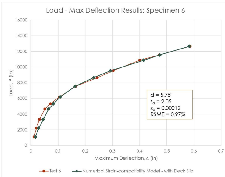
Fig. 4.26(e) Load-deflection model comparison with test specimen 6.
