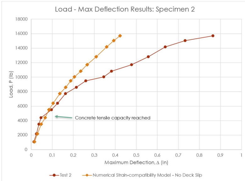
Fig. 4.22(a) Load-deflection model with no slip comparison with test specimen.
