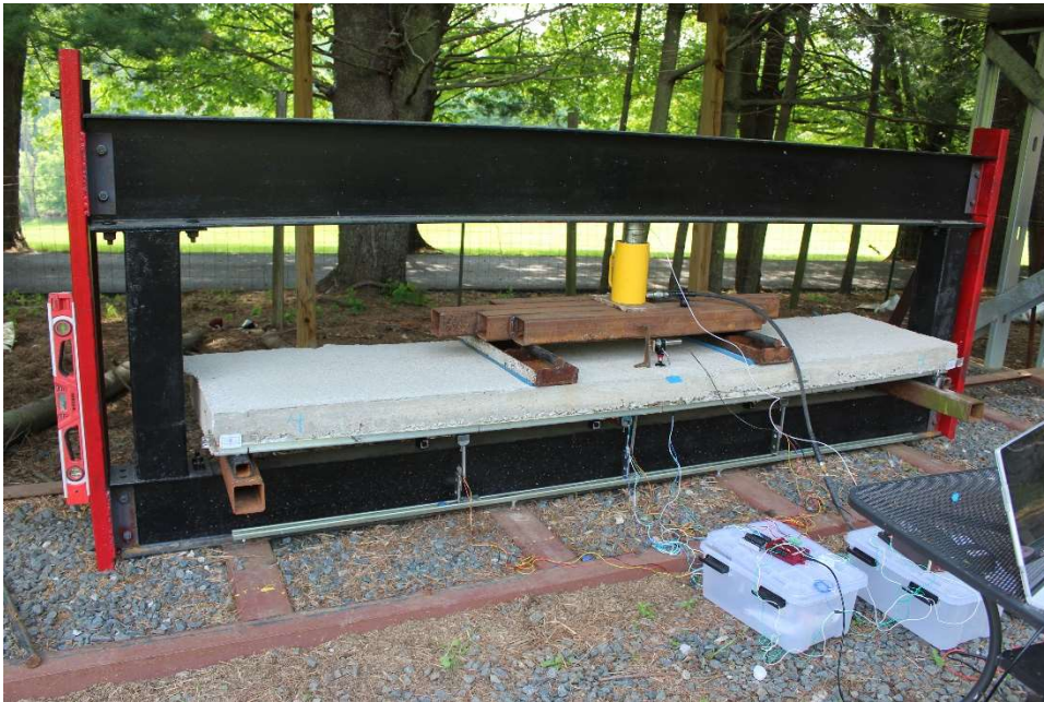
Fig. 3.3 Load frame apparatus with specimen loaded and sensors installed.
