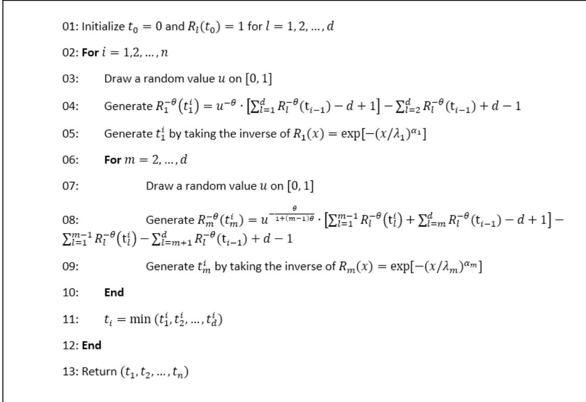
Figure 4-9: Pseudo-code of the series system's failure times generating algorithm
