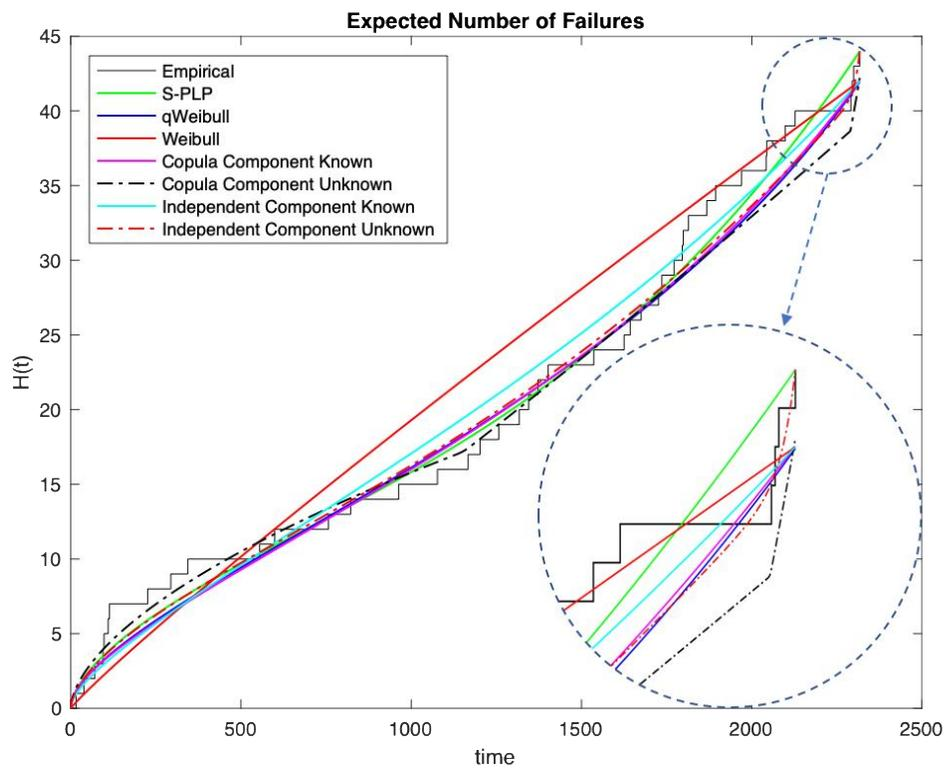
Figure 4-13: Comparison of cumulative intensity for LHD machine failures
