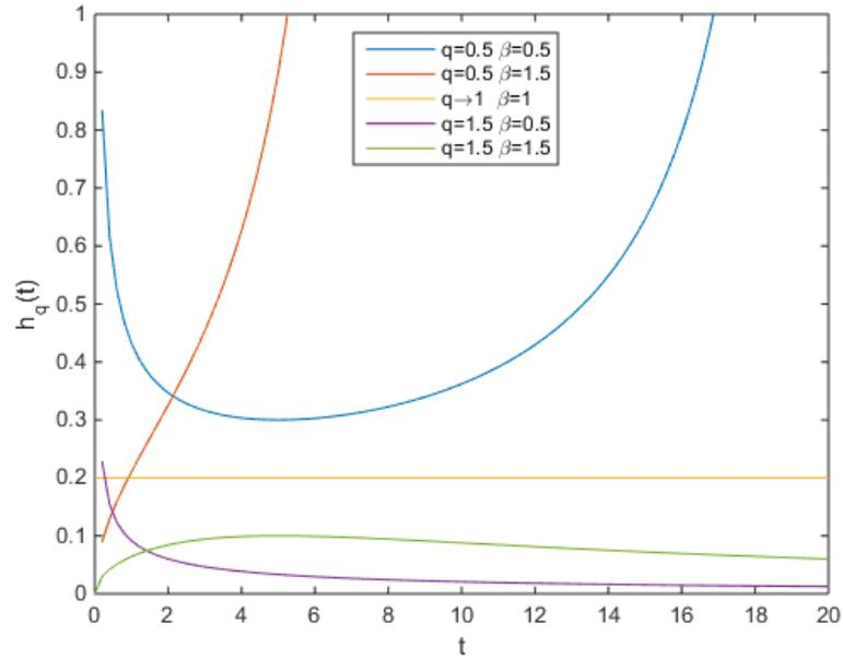
Figure 2-1: Behaviors of the q-Weibull hazard rate function for  $\eta = 5$  and different values of the shape parameters  $q$  and  $\beta$
