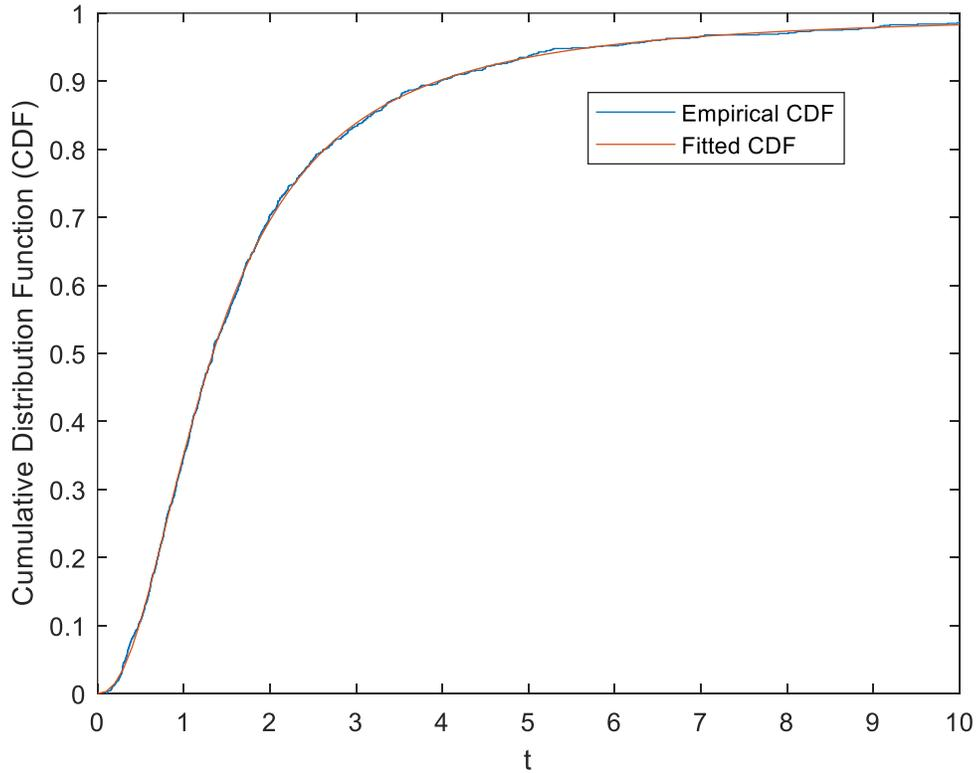
Figure 5-7: Comparison of the empirical and fitted CDFs of the system’s lifetime.
