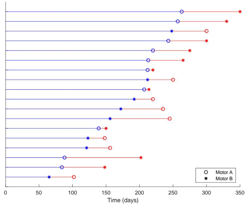
Figure 5-3: Times to failure (in days) for two motors.
