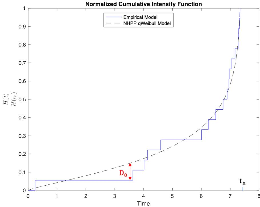
Figure 4-10: The normalized empirical and fitted cumulative intensity function and the illustration of  $D_0$
