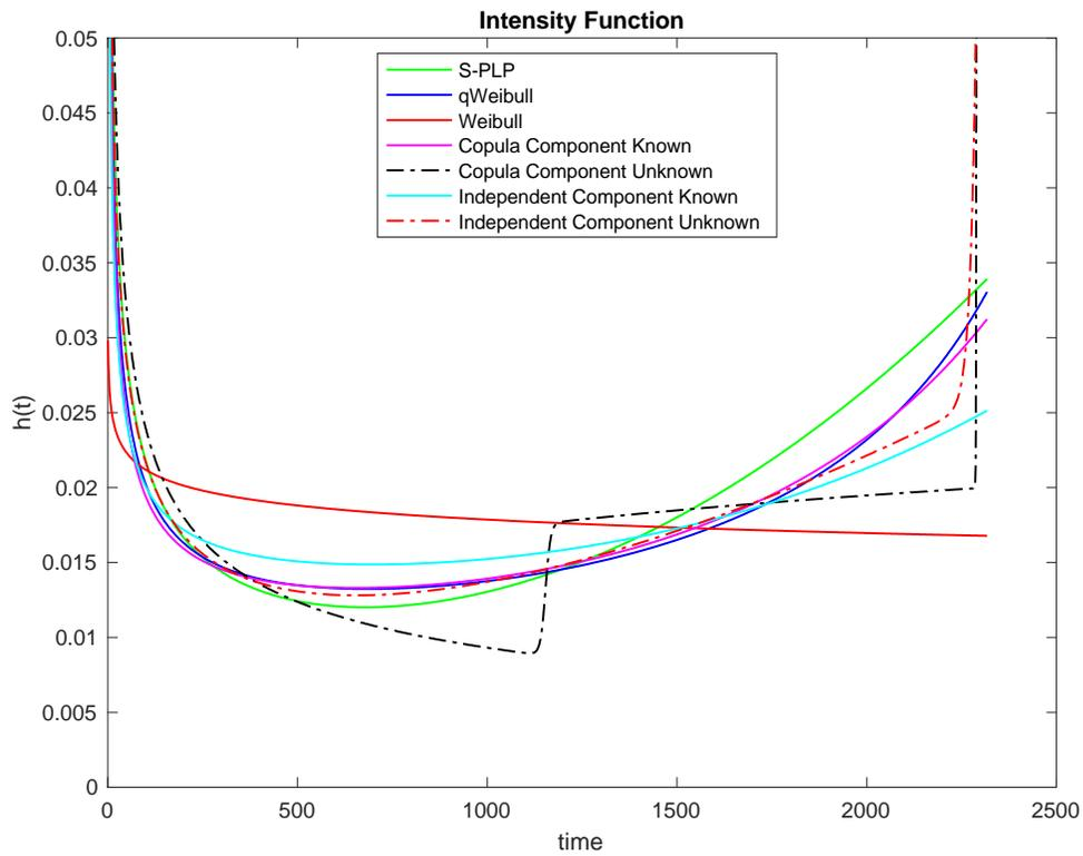
Figure 4-14: Comparison of intensity functions for LHD machine failures
