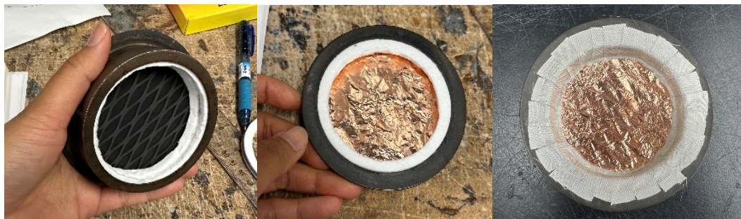
Figure A1.2. Sample holder for FPUF samples used in CAPA II experiment.
