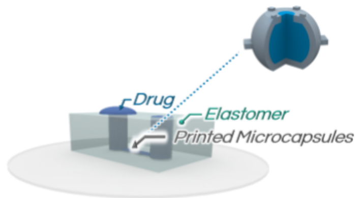
Figure 3-5. Loading of the liquid core into the microcapsule using PDMS microchannel. [14]
