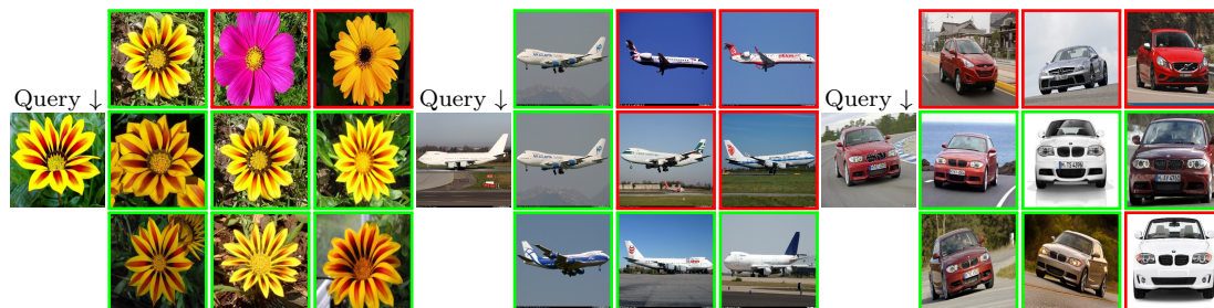
Figure 5.9: Retrieval qualitative evaluation on three FGVR datasets: Flowers-102, Aircrafts and Cars. Given a query image, the three nearest neighbors are depicted. The three consecutive rows show search results using center loss, semi-hard and hard triplet regularizers. Green and red outlines denote match and mismatch between the query and its result respectively.
