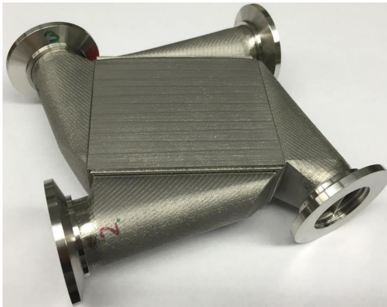
Figure 8-12: Test section including core, headers, and flanges before welding
