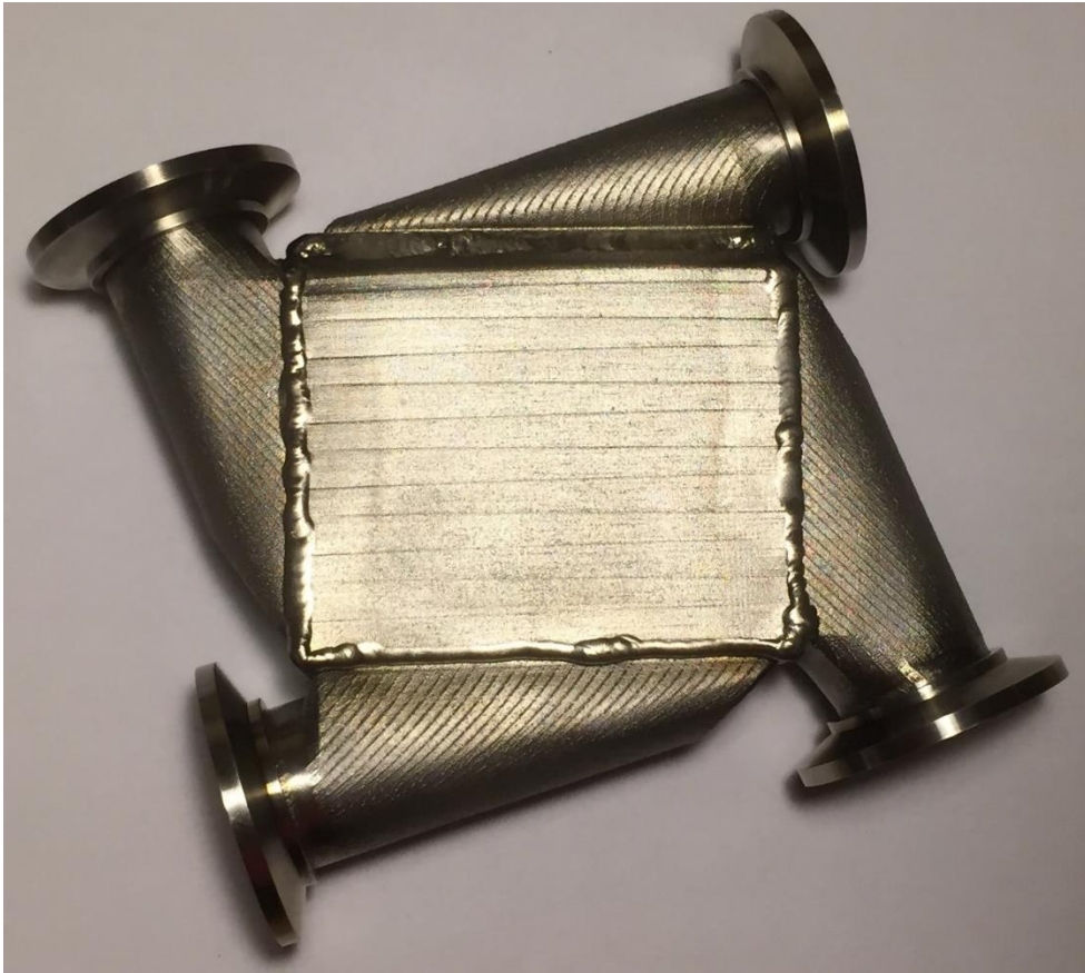
Figure 8-13: Welded test section including core, headers, and flanges
