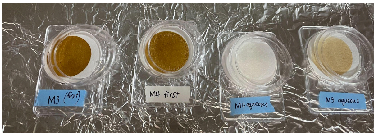
Figure 29: Sediment-Clogged Slides Which did not Receive Density Separation
