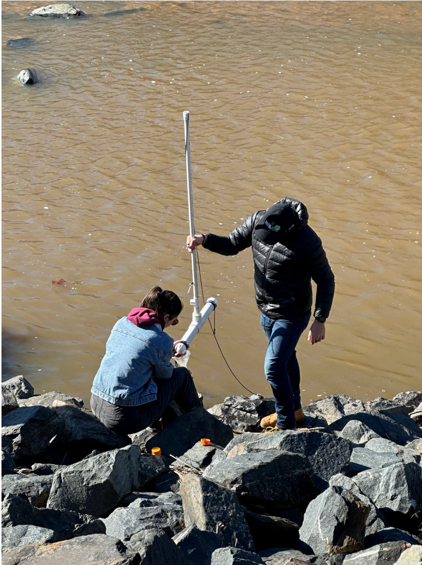
Figure 27: Apparatus Being Used to Collect a 1 L Sample
