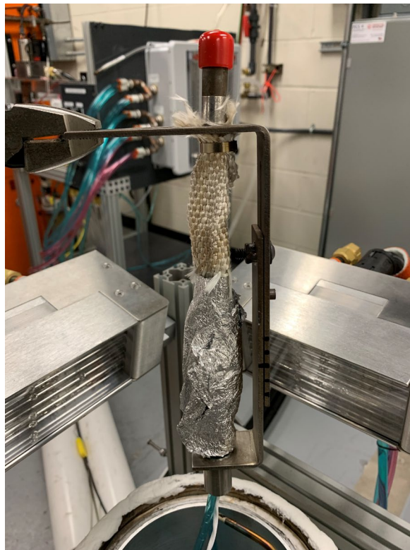
Figure 2.23: Heat Flux Gauge Mount with Heat flux gauge installed.
