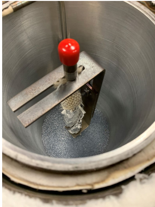
Figure B.18: Heat flux gauge mounted in air distribution chamber fitting.
