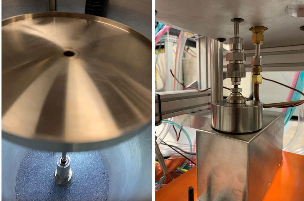
Figure B.24: Sample holder through the bearing with the adjustable base foot installed.
