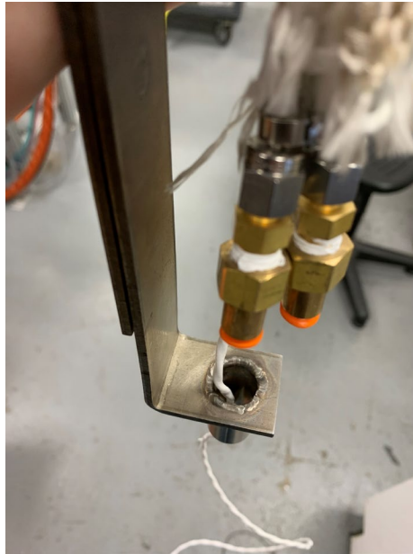
Figure B.13: Heat flux gauge sensor wires run through mount center passthrough.
