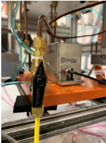
Figure B.33: Pilot flame downstream valve in the on position.
