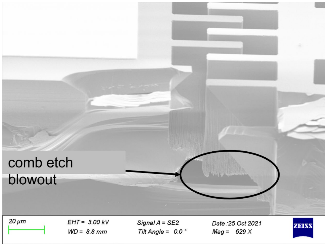
Figure 2.4-11. Example of feature blowout at the comb location near the buried oxide. The lateral etch rate behavior of the PlasmaTherm provided “Finishing Etch” caused 5 \mu\text{m} to lose 15-25 \mu\text{m} of total height.
