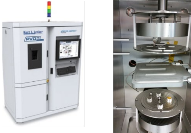
Figure 3.1-3. Custom high vacuum packaging furnace developed as collaborative effort between the author, researchers at the US Army Research Laboratory (ARL), and the Kurt J. Lesker Company.
