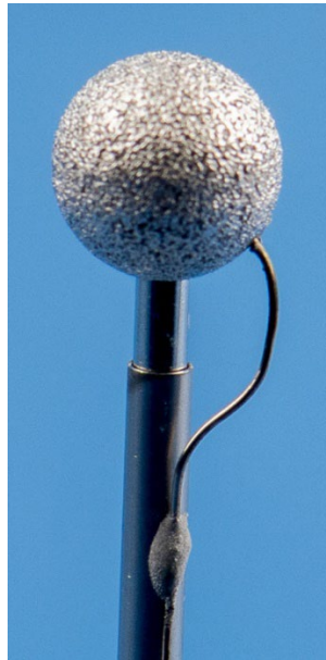
Fig. 2.2. 6.4 mm diameter spherical burner used for microgravity experiments. A 0.25 mm type-K thermocouple is embedded in the burner surface.
