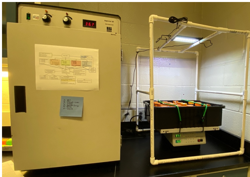
Figure 2.3. Experimental set-up for Trial #1 and #2. The bottles were placed on the orbital shaker (right) with a light place on top with the incubator (left) used for microbial enumeration analysis.
