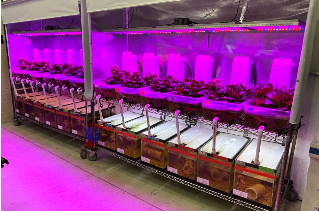
Figure 3.2. Picture of the 12 aquaponic systems used in Phase 1 and 2. Each system contained a fish tank with 4 goldfish, grow bed with 4 plants (2 basil and 2 lettuce), 3-tier biofiltration system and LED lights.
