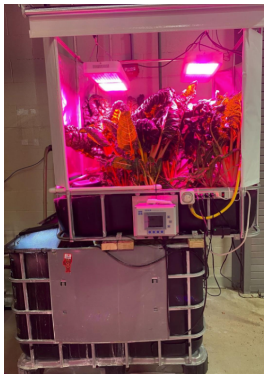
Figure 2.2. The 1040 L parent aquaponic system (IBC) that had been continuously operating for 3 years. All aquaponic effluent used in preliminary experiment Trial #1 and #2 were collected from this system due to its established microbial community.
