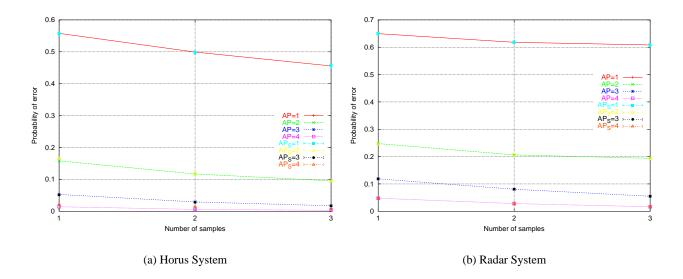
Figure 3. Probability of error for the *Horus* and *Radar* systems under a uniform user profile (profile 1).
