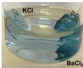
Figure 4.11: Qualitative dye uptake experiments show 8AmG/G-KCl vs 8AmG/G-BaCl 2 gels after soaking in 12.5μM NBB 36 for 24 hours. While 8AmG/G-KCl gels will absorb NBB 36 from solution, 8AmG/G-the BaCl 2 gels absorbs the dye much faster. 17
