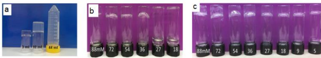
Figure 3.2: a) Samples of hydrogels with 50.0 of mg G 1 in various amounts of water (indicated on vials). BDBA-K, 59 mM G 1 (left), BDBA-Ba, 18mM G 1 (middle) and 4mM G 1 , BDBA-Mg (right). b) BDBA-K gels of varying G 1 concentrations (from 88 to 18 mM, as indicated on vials) made with G 1 :BDBA 4 :KOH = 1:0.5:1 c) BDBA-Mg gels of varying concentrations of G 1 (from 88 to 5 mM, as indicated on vials), made by preforming a BDBA-K gel and diluting with H 2 O, then adding 5 mM Mg 2+ . 16
