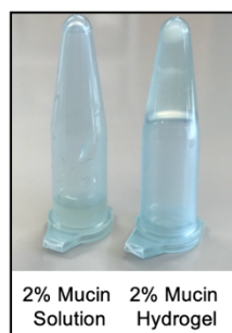
Figure 2.8 Inversion test to confirm gelation. 2% mucin solution (left) and 2% mucin hydrogel that used 2% thiolated PEG polymer (right).
