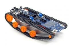
Figure 3.1: Arduino fitted with tank treads, purchased from Robot Shop.
